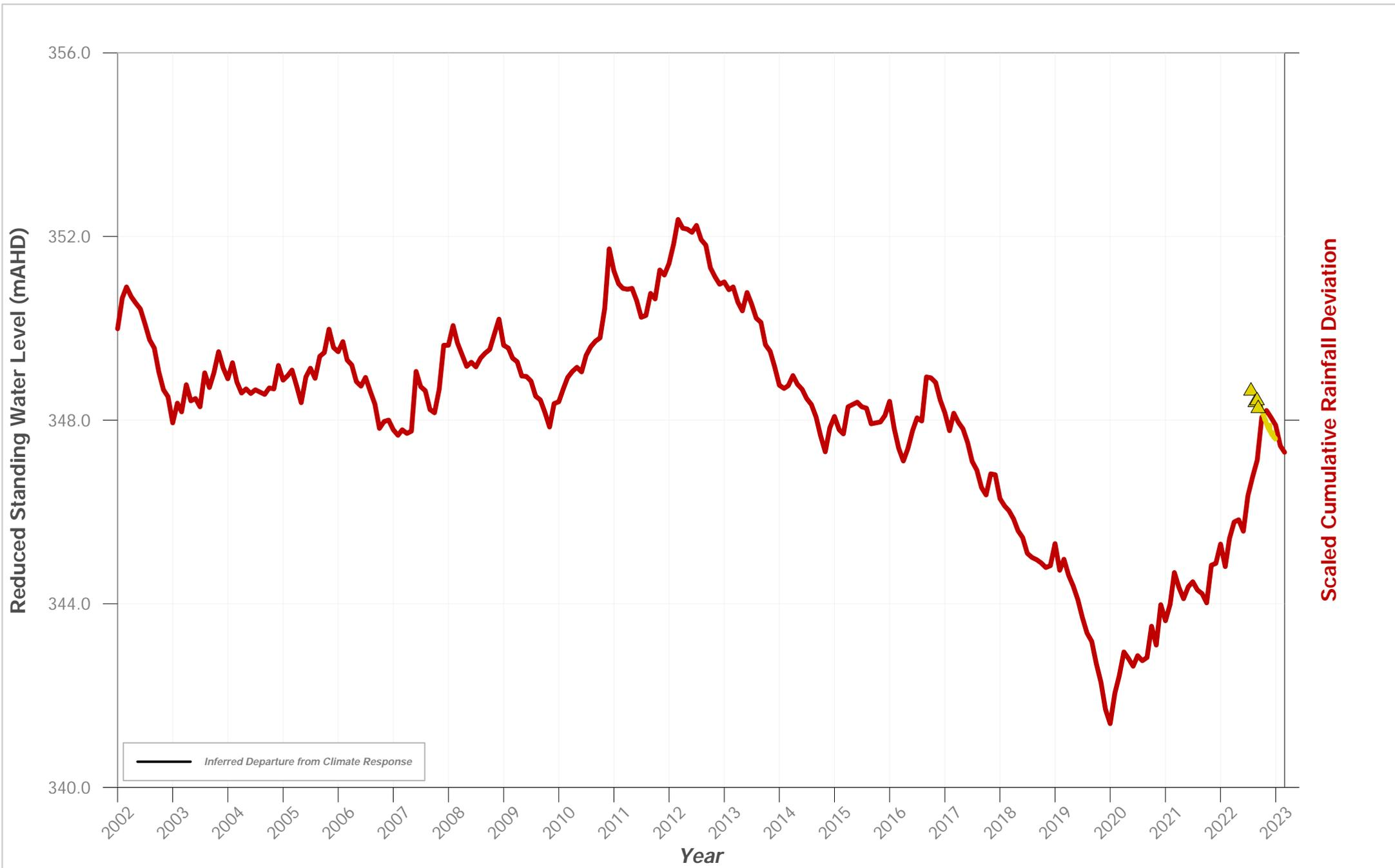
**Hydrograph of Groundwater Level Data for Bore ID: PZ 103D VWP 85m**
