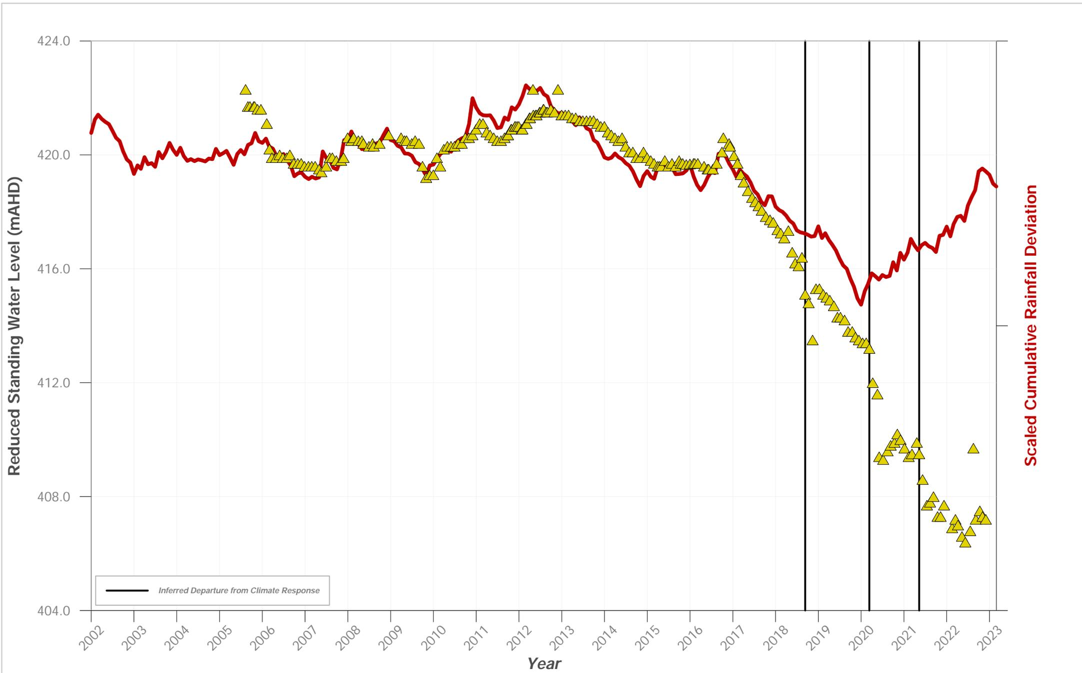
**Hydrograph of Groundwater Level Data for Bore ID: PZ 040B**
