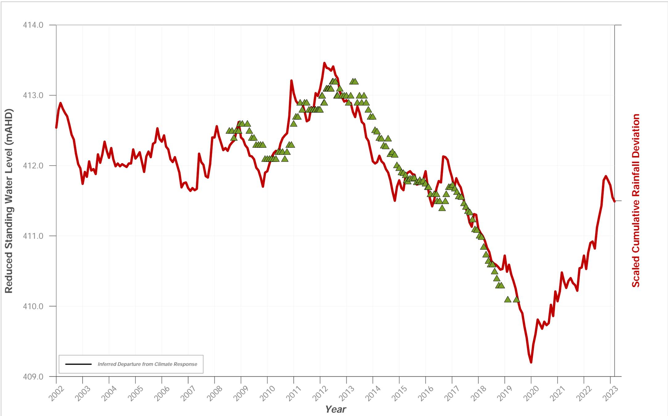
**Hydrograph of Groundwater Level Data for Bore ID: PZ 184**
