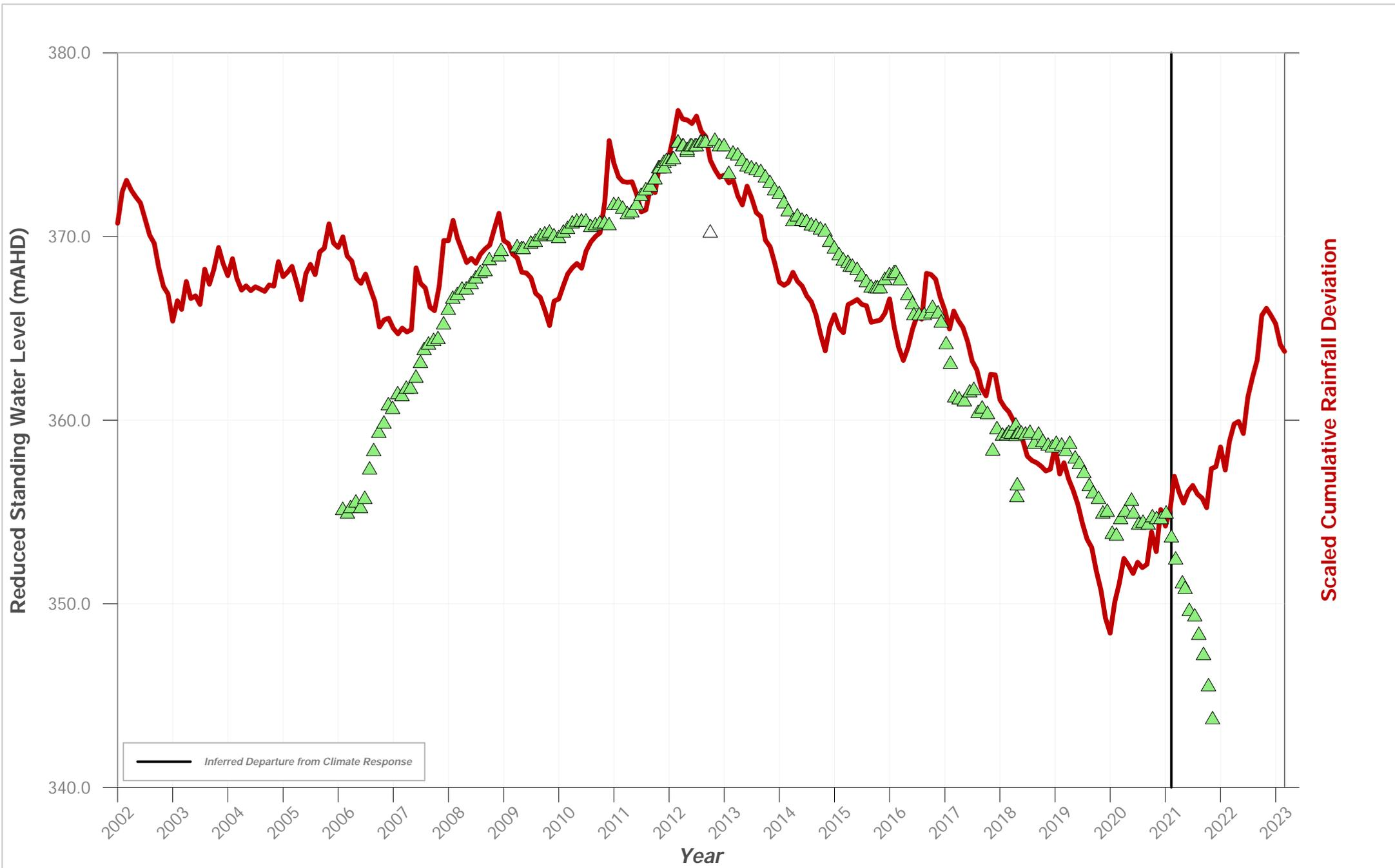
**Hydrograph of Groundwater Level Data for Bore ID: PZ 102B**
