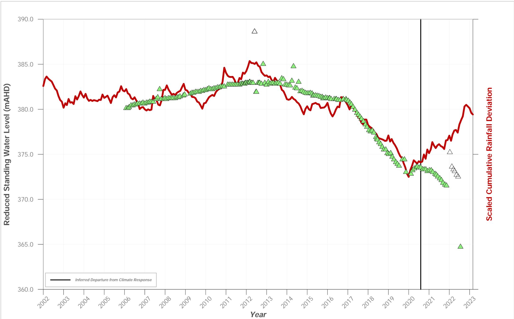
**Hydrograph of Groundwater Level Data for Bore ID: PZ 104**
