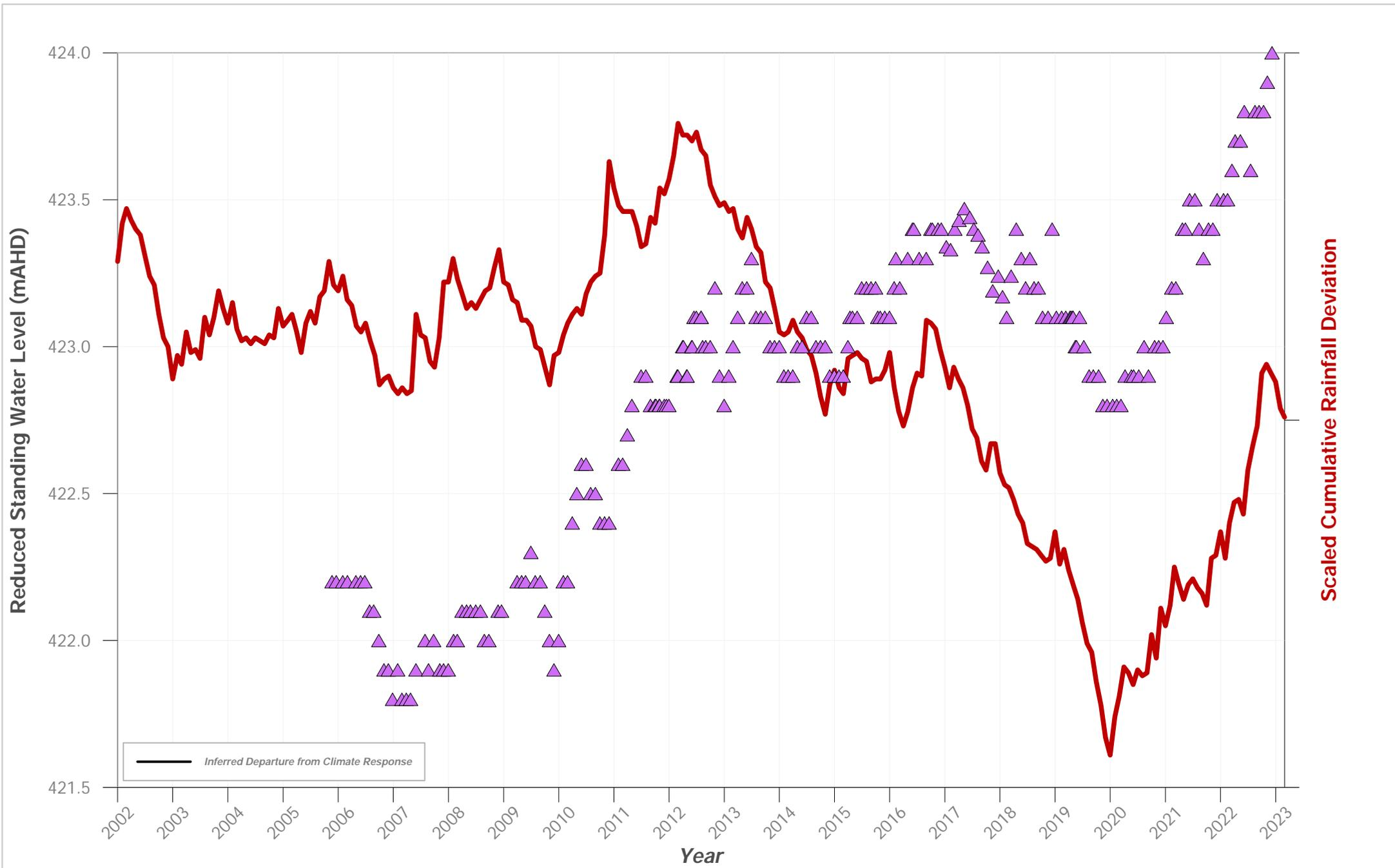
**Hydrograph of Groundwater Level Data for Bore ID: PZ 055**
