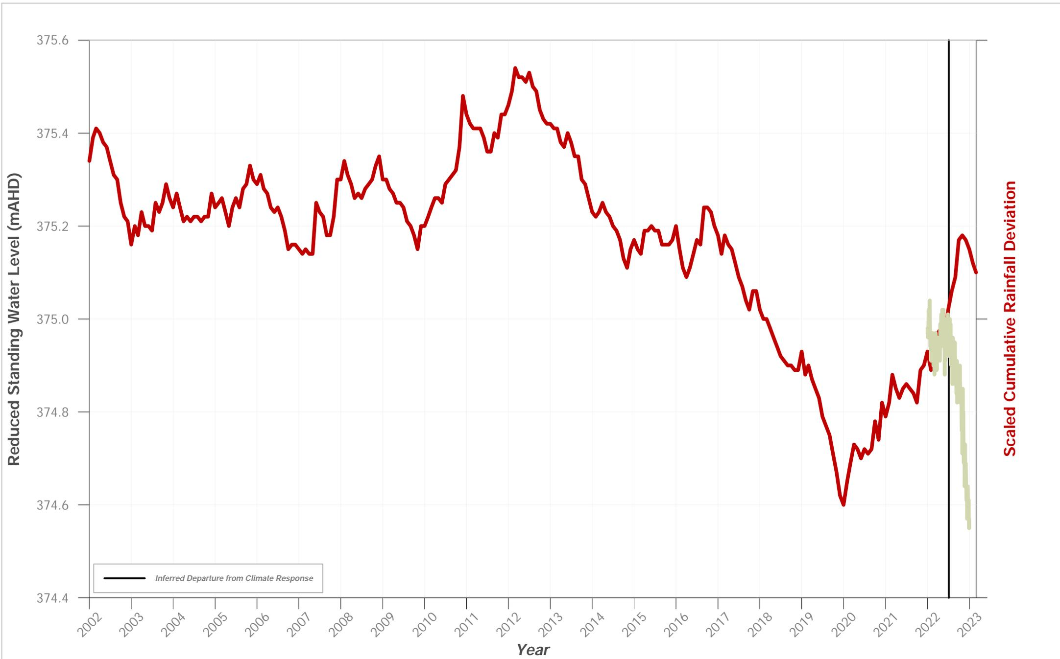
**Hydrograph of Groundwater Level Data for Bore ID: PZ 230 VWP 130m**
