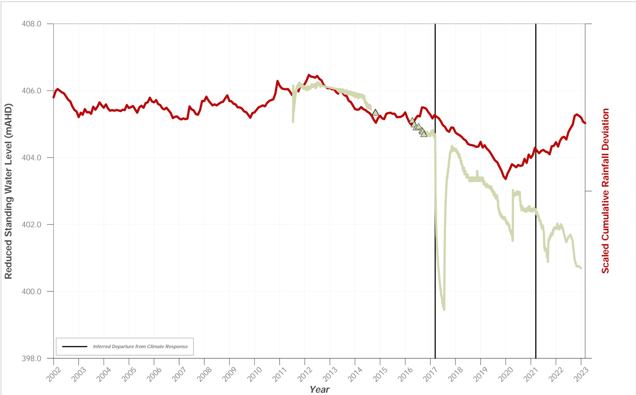
**Hydrograph of Groundwater Level Data for Bore ID: PZ 192 VWP 68m**
