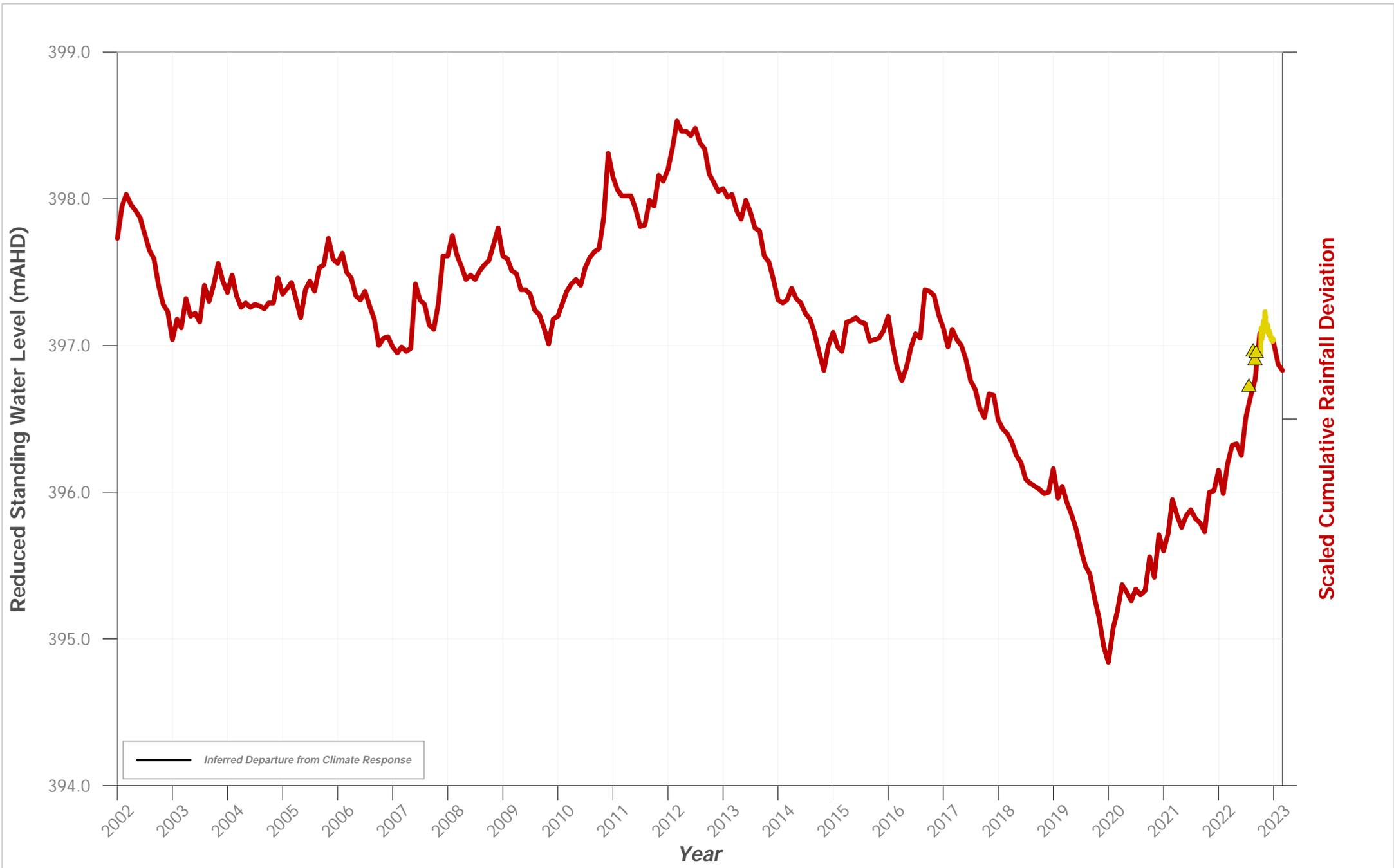
**Hydrograph of Groundwater Level Data for Bore ID: PZ 103D VWP 31m**
