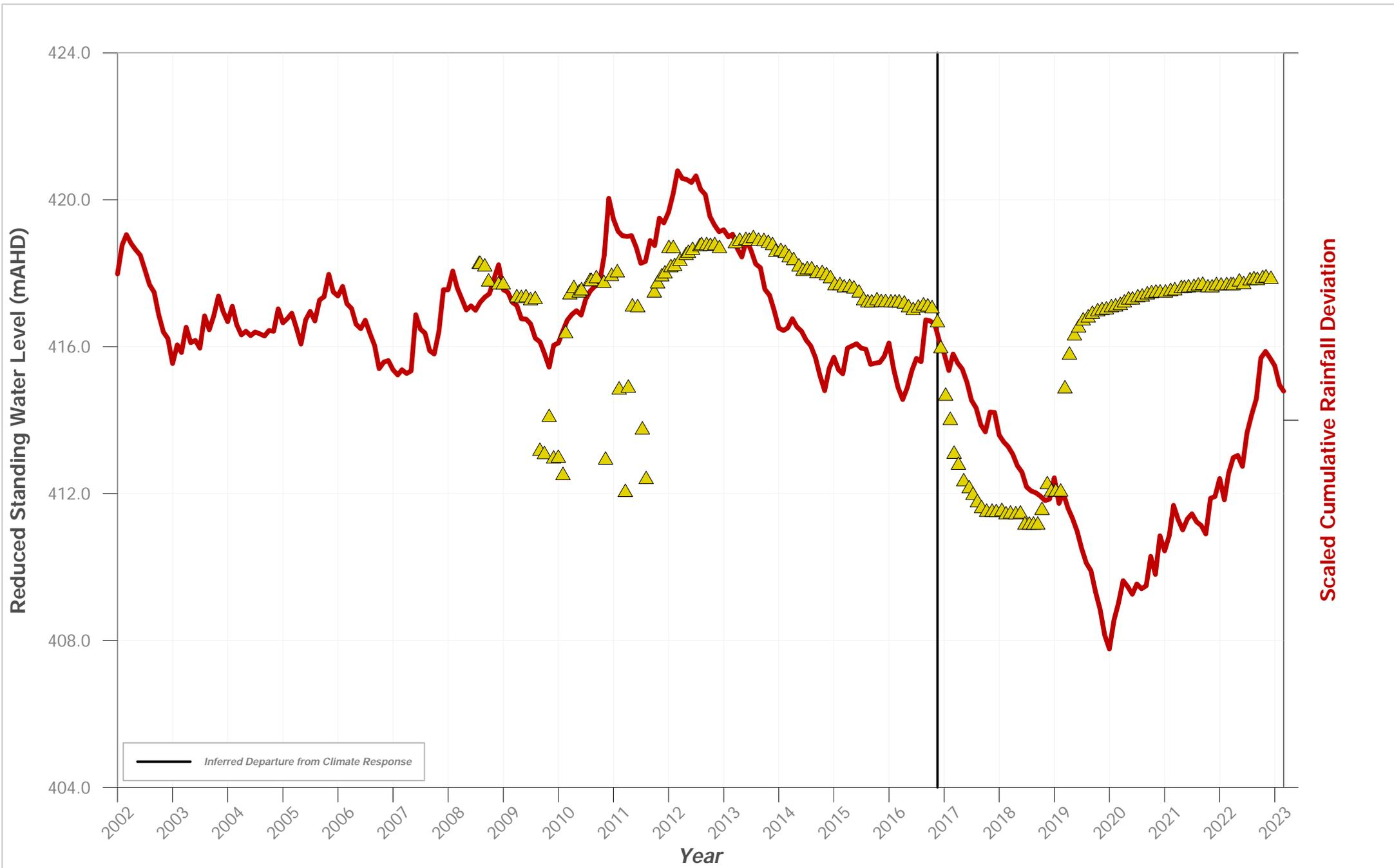
**Hydrograph of Groundwater Level Data for Bore ID: PZ 179 VWP 33m**
