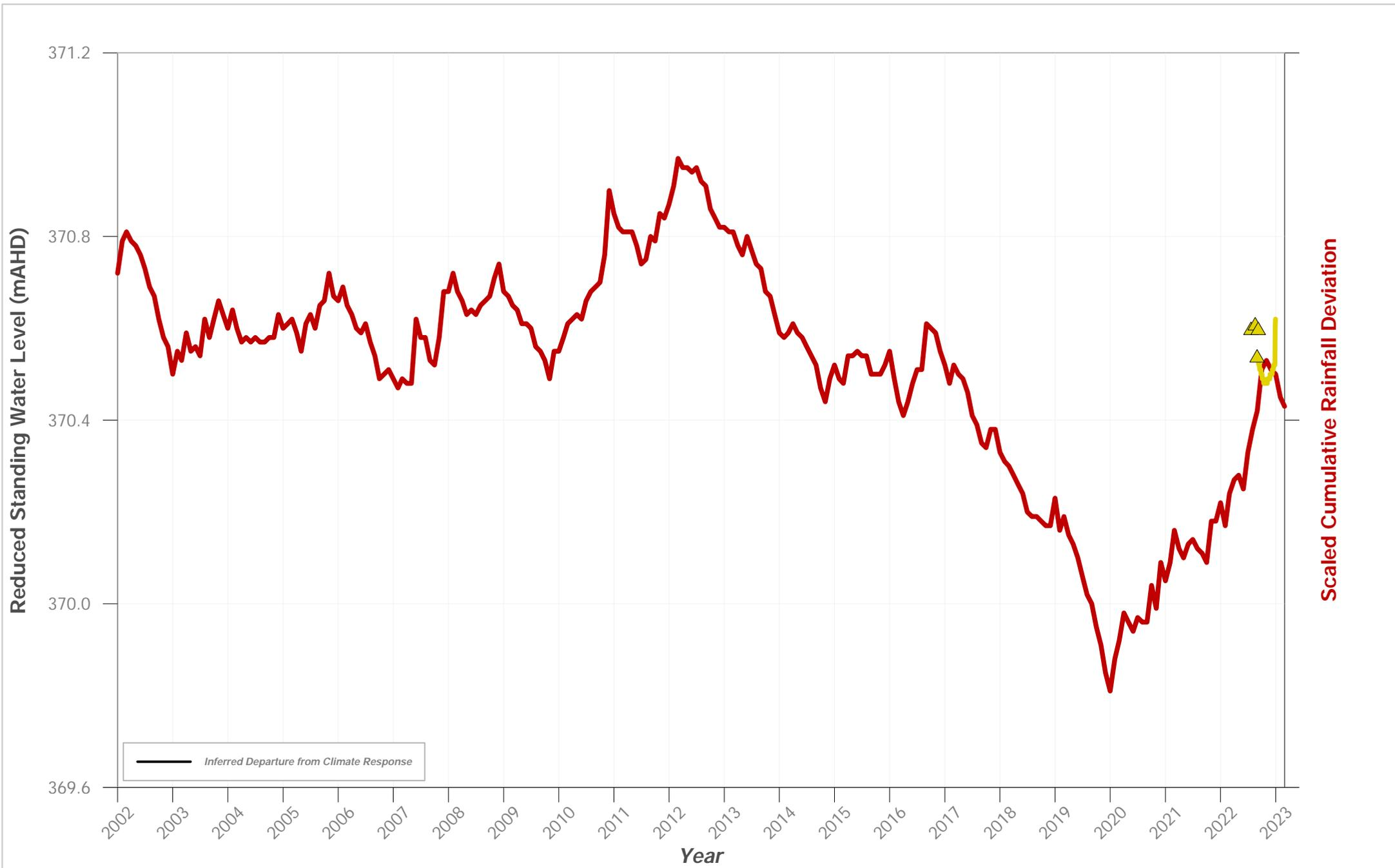
**Hydrograph of Groundwater Level Data for Bore ID: PZ 103D VWP 55m**
