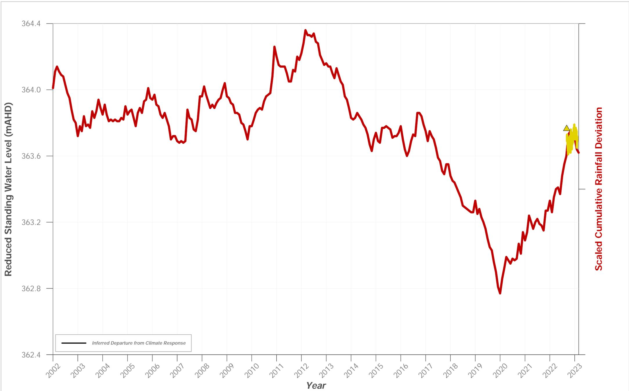
**Hydrograph of Groundwater Level Data for Bore ID: PZ 232 VWP 132m**
