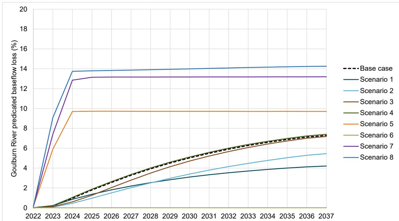
Figure 8.19 Modelled Baseflow Reduction due to LW401-408
