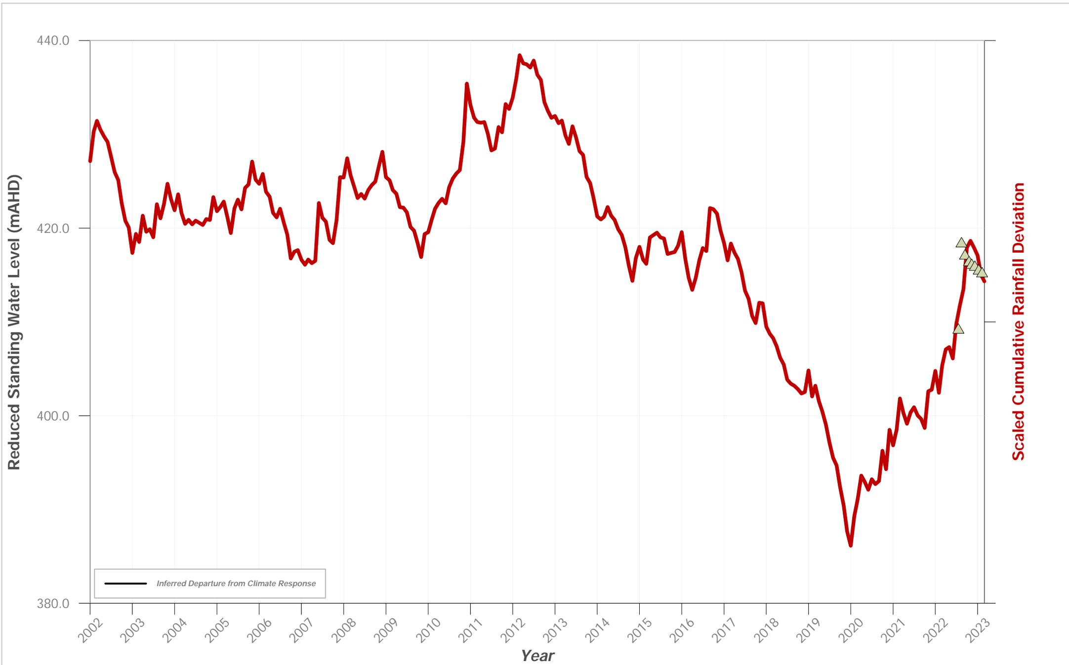
**Hydrograph of Groundwater Level Data for Bore ID: PZ 194B**
