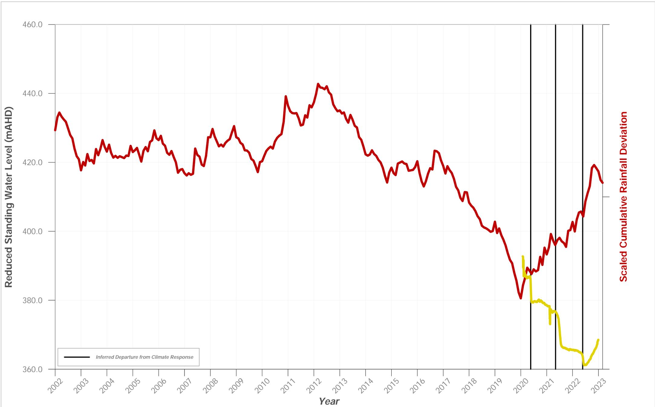
**Hydrograph of Groundwater Level Data for Bore ID: PZ 186 VWP 65m**
