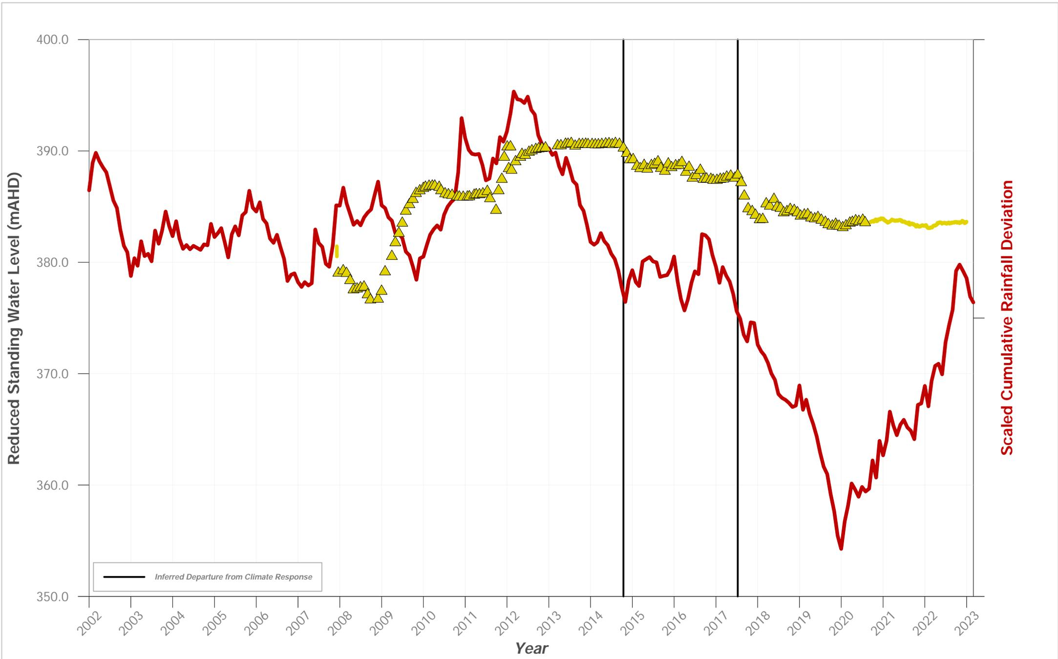
**Hydrograph of Groundwater Level Data for Bore ID: PZ 129 VWP 53m**
