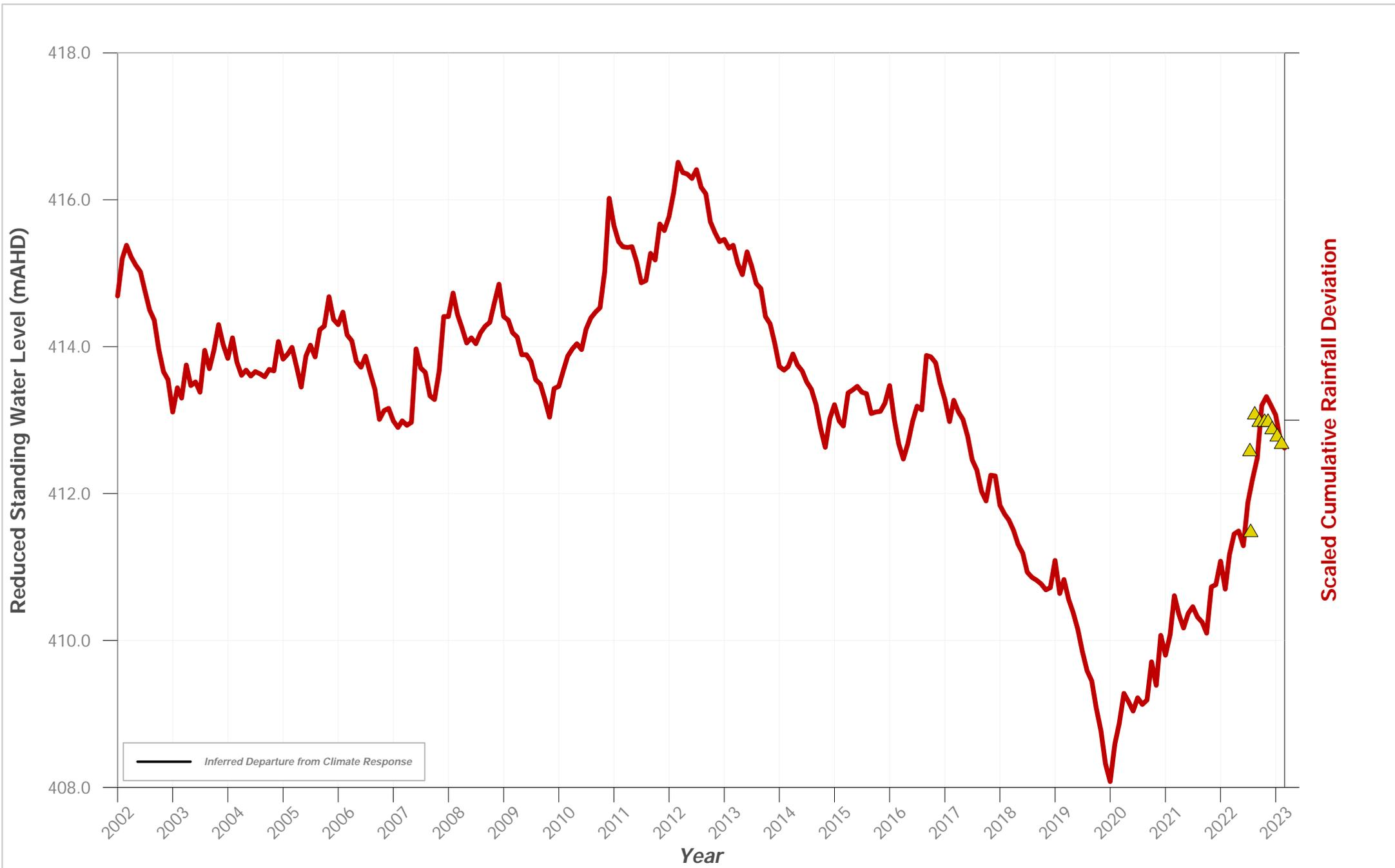
**Hydrograph of Groundwater Level Data for Bore ID: PZ 194C**
