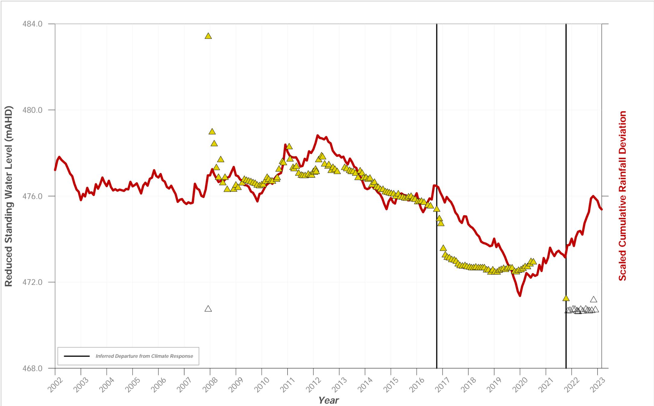
**Hydrograph of Groundwater Level Data for Bore ID: PZ 130 VWP 64m**
