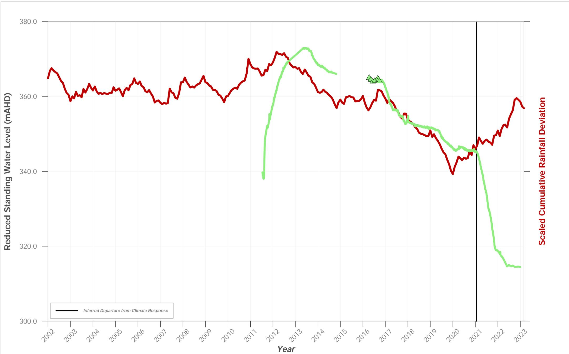
**Hydrograph of Groundwater Level Data for Bore ID: PZ 192 VWP 178m**
