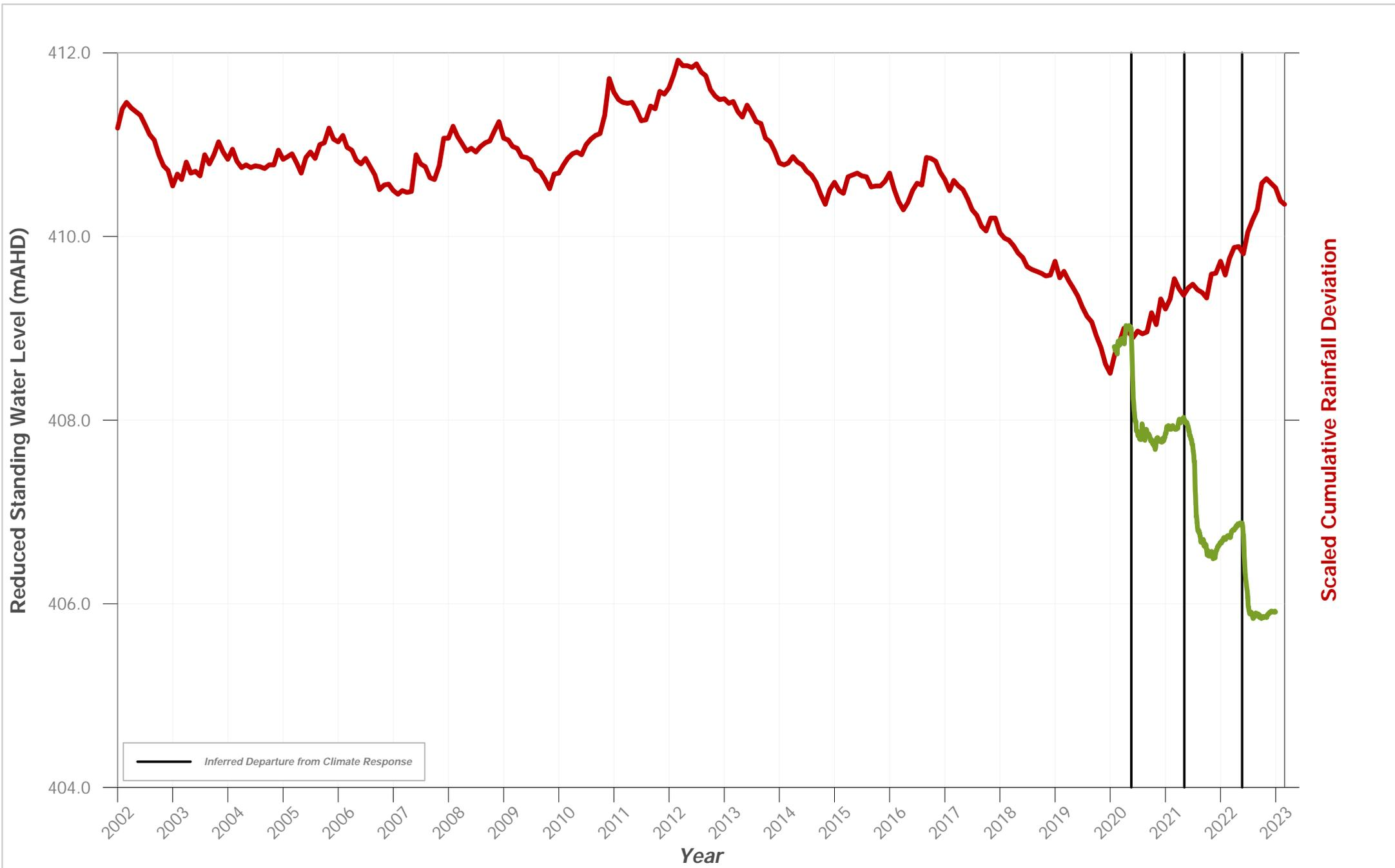
**Hydrograph of Groundwater Level Data for Bore ID: PZ 186 VWP 13.5m**
