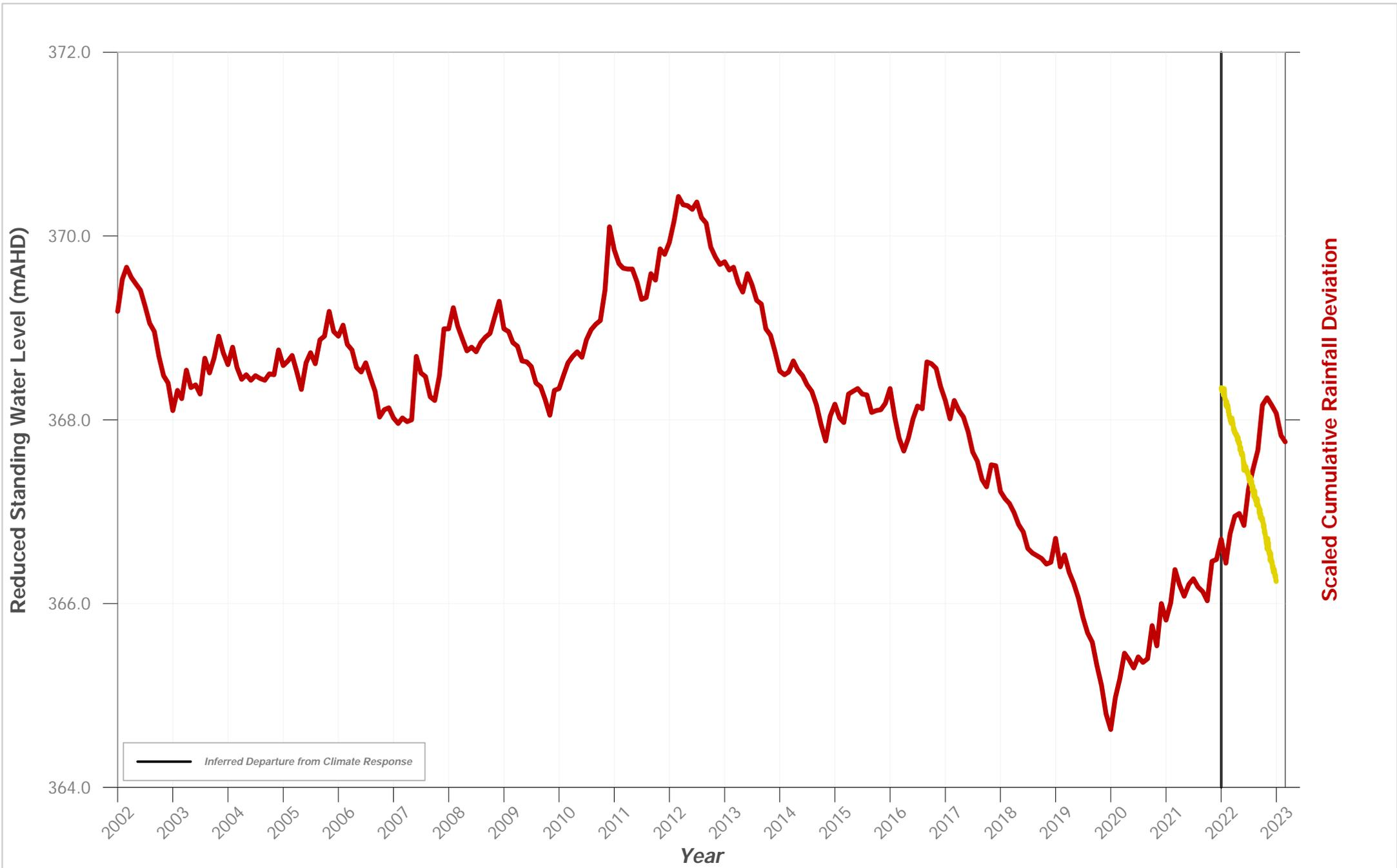
**Hydrograph of Groundwater Level Data for Bore ID: PZ 230 VWP 187m**
