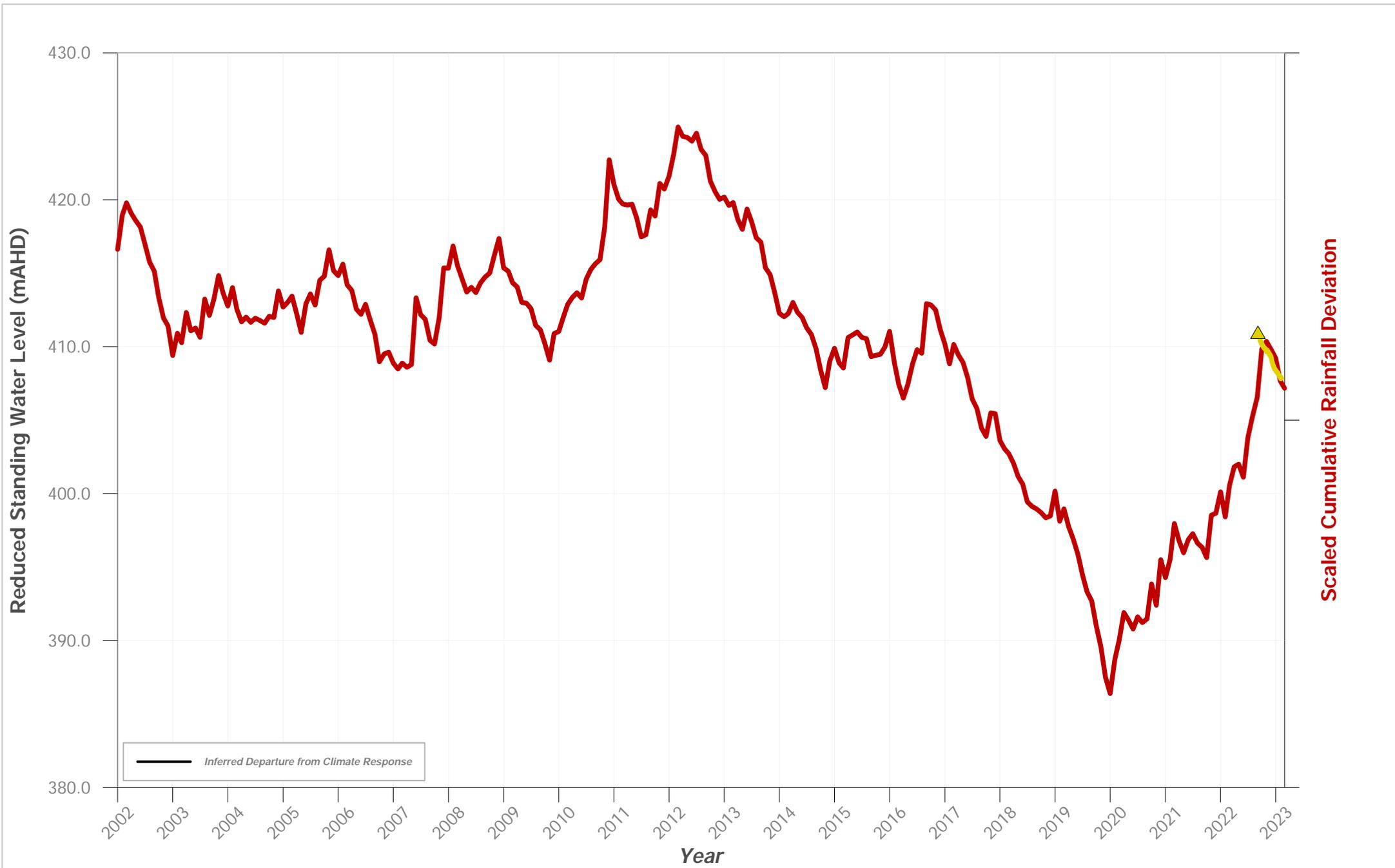
**Hydrograph of Groundwater Level Data for Bore ID: PZ 232 VWP 96m**
