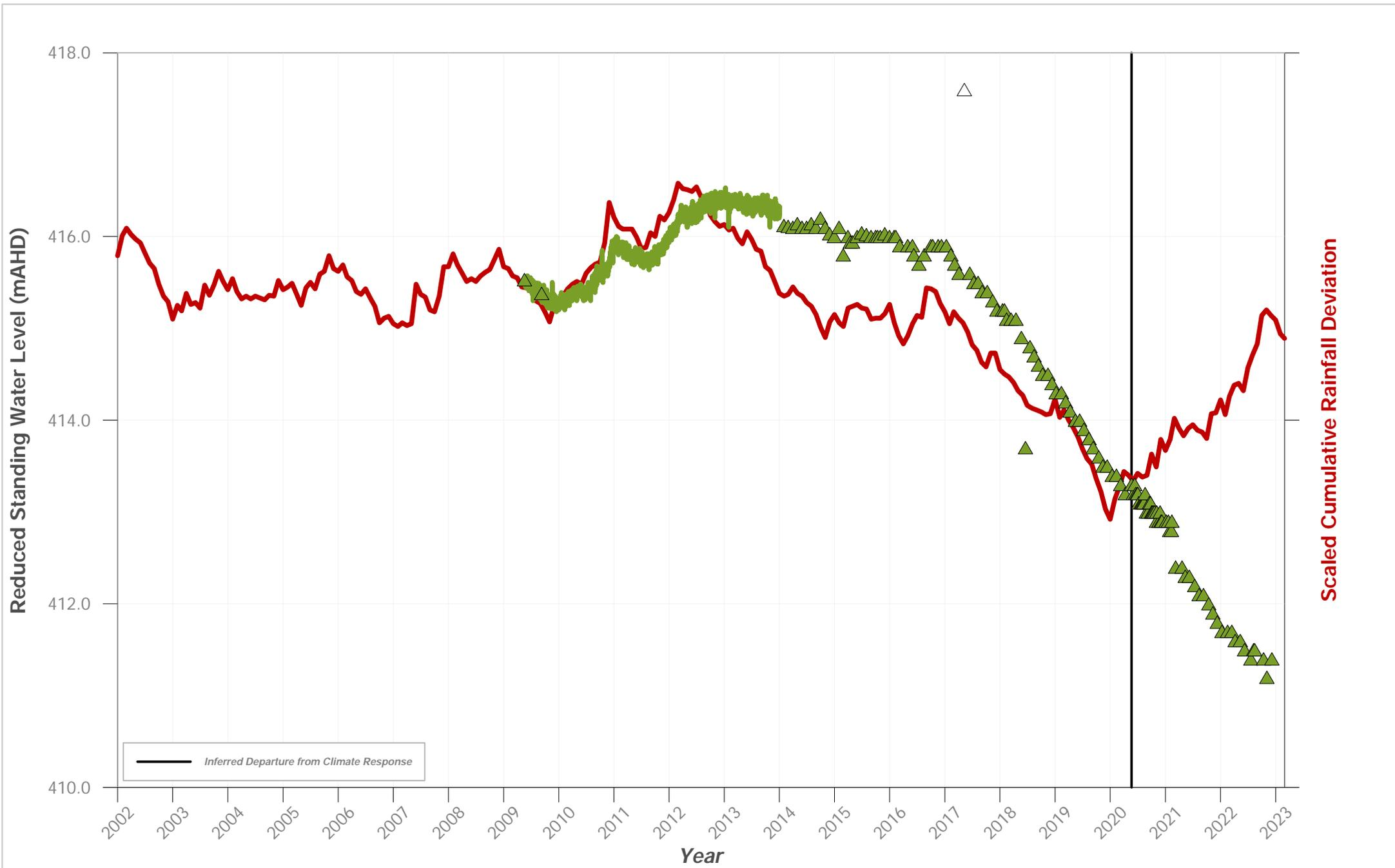
**Hydrograph of Groundwater Level Data for Bore ID: PZ 188**
