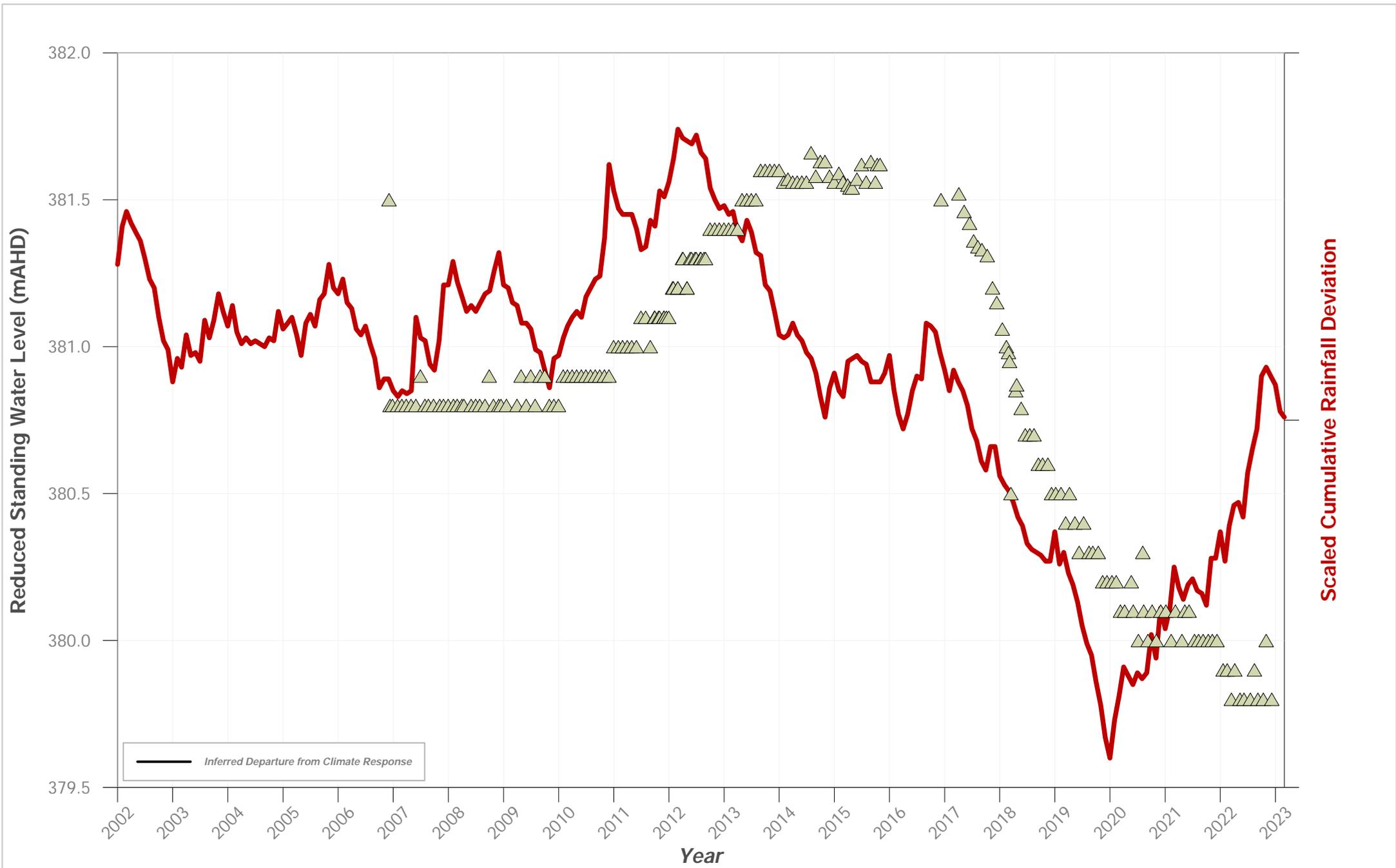
**Hydrograph of Groundwater Level Data for Bore ID: PZ 101C**
