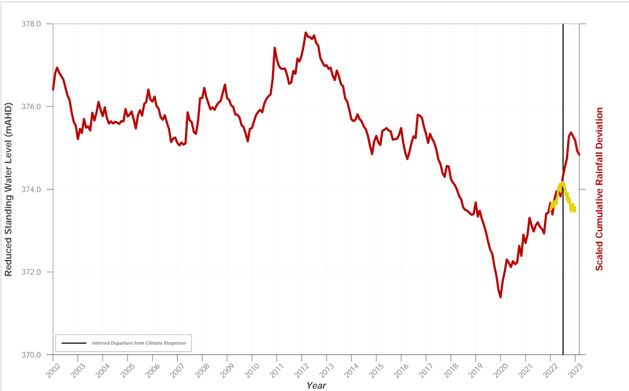
**Hydrograph of Groundwater Level Data for Bore ID: PZ 229 VWP 316m**
