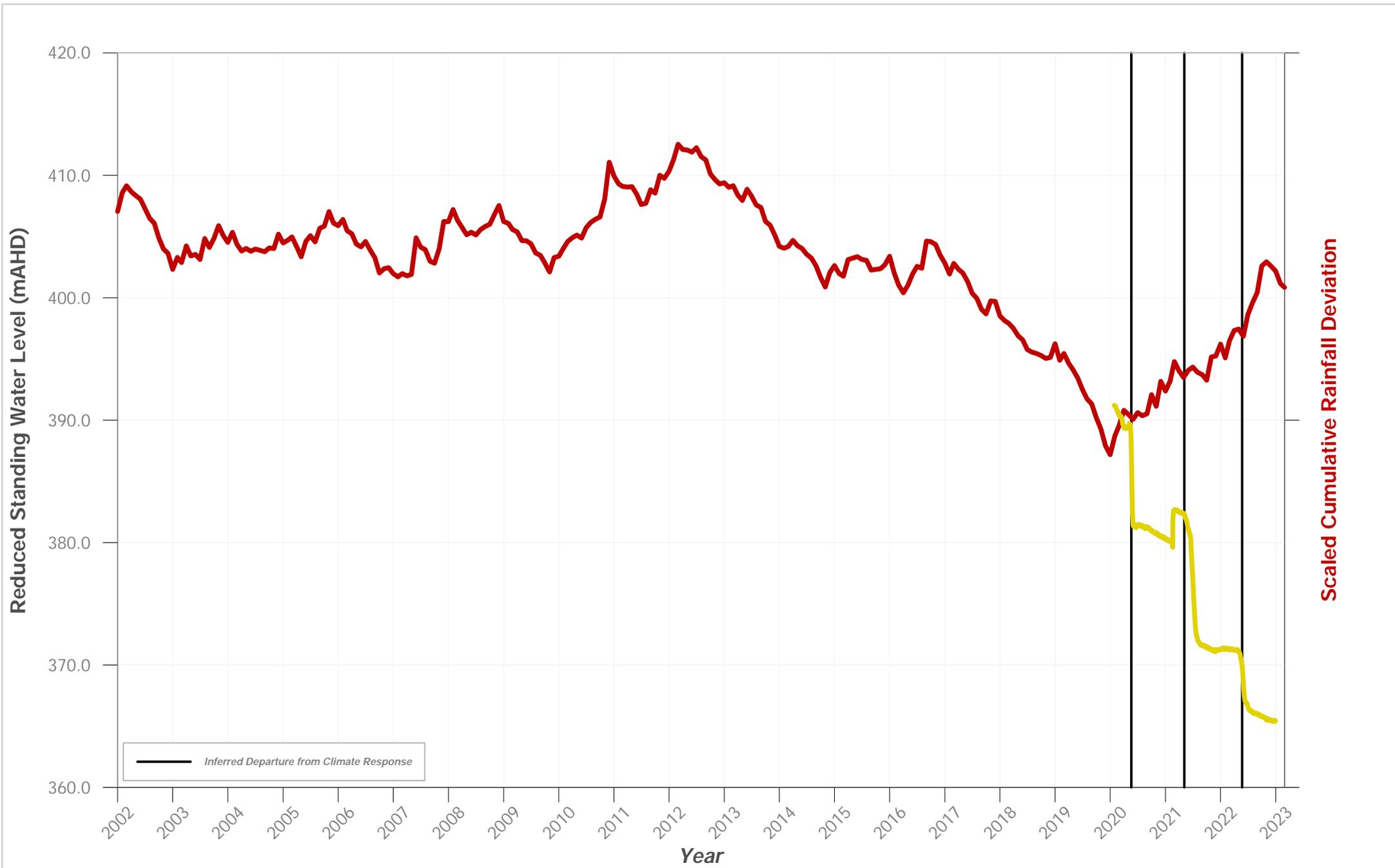
**Hydrograph of Groundwater Level Data for Bore ID: PZ 186 VWP 86m**
