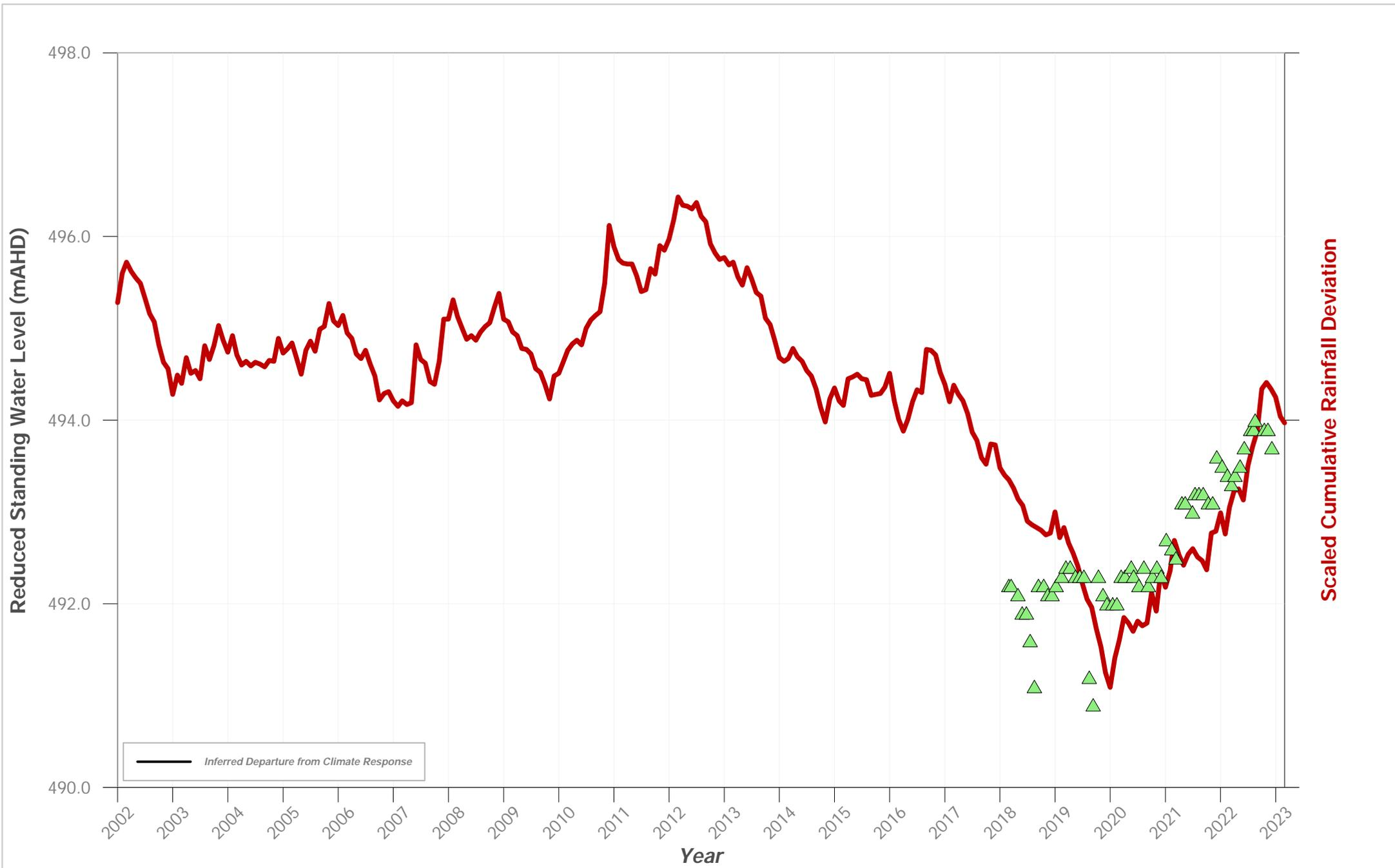
**Hydrograph of Groundwater Level Data for Bore ID: PZ 217**
