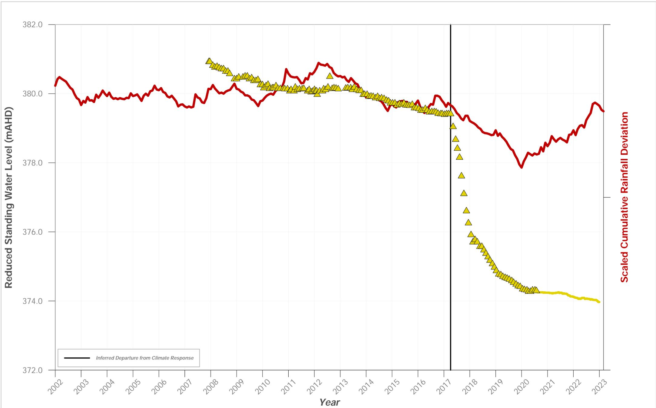
**Hydrograph of Groundwater Level Data for Bore ID: PZ 128 VWP 36m**
