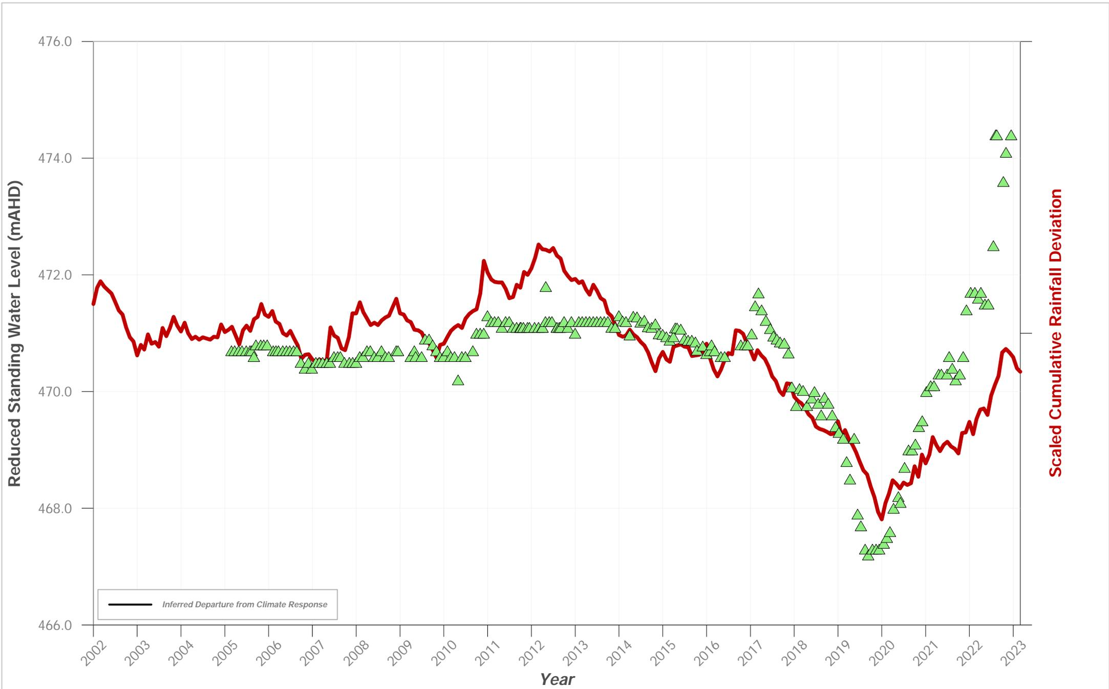
**Hydrograph of Groundwater Level Data for Bore ID: PZ 003**
