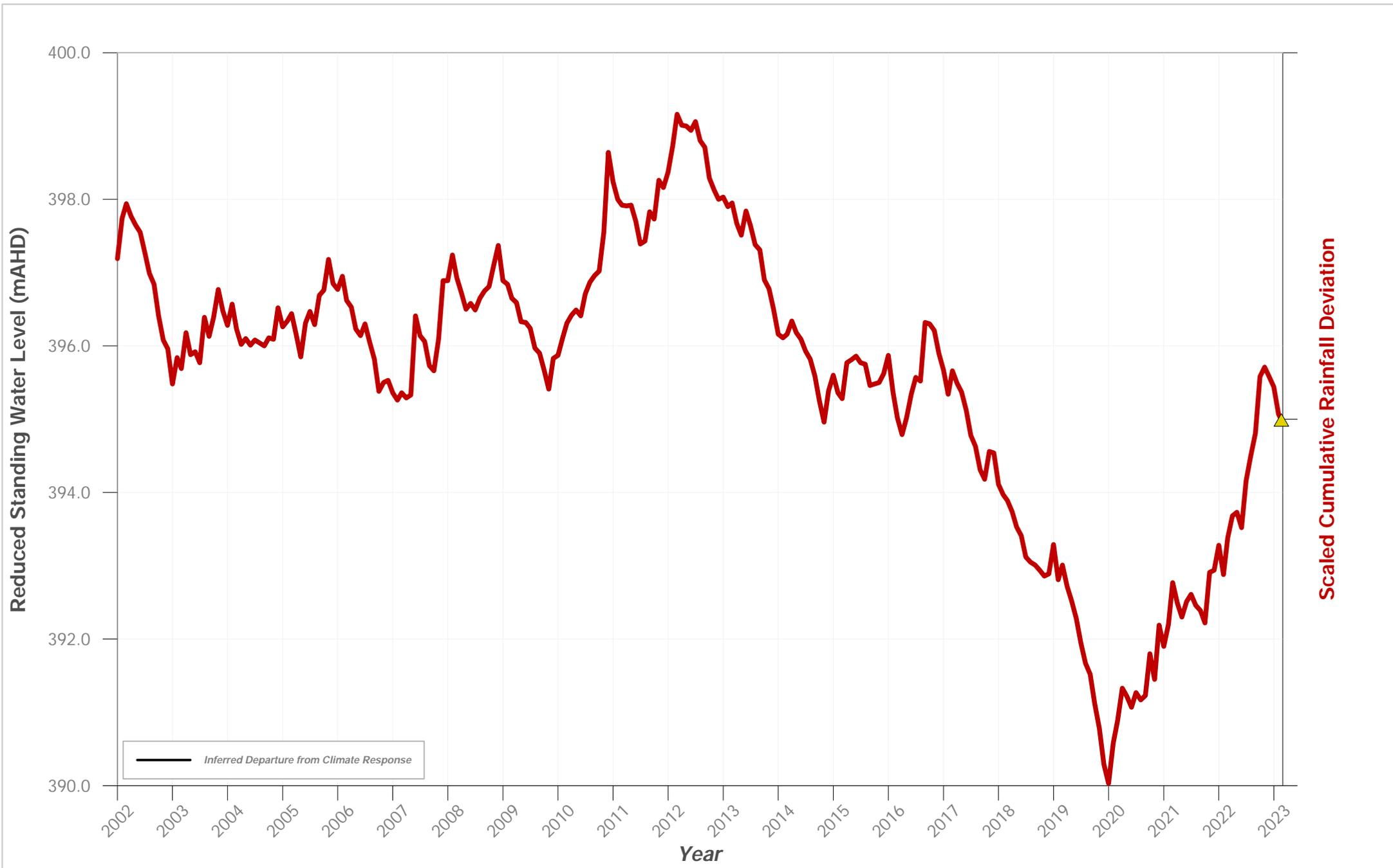
**Hydrograph of Groundwater Level Data for Bore ID: PZ 238 VWP 50m**
