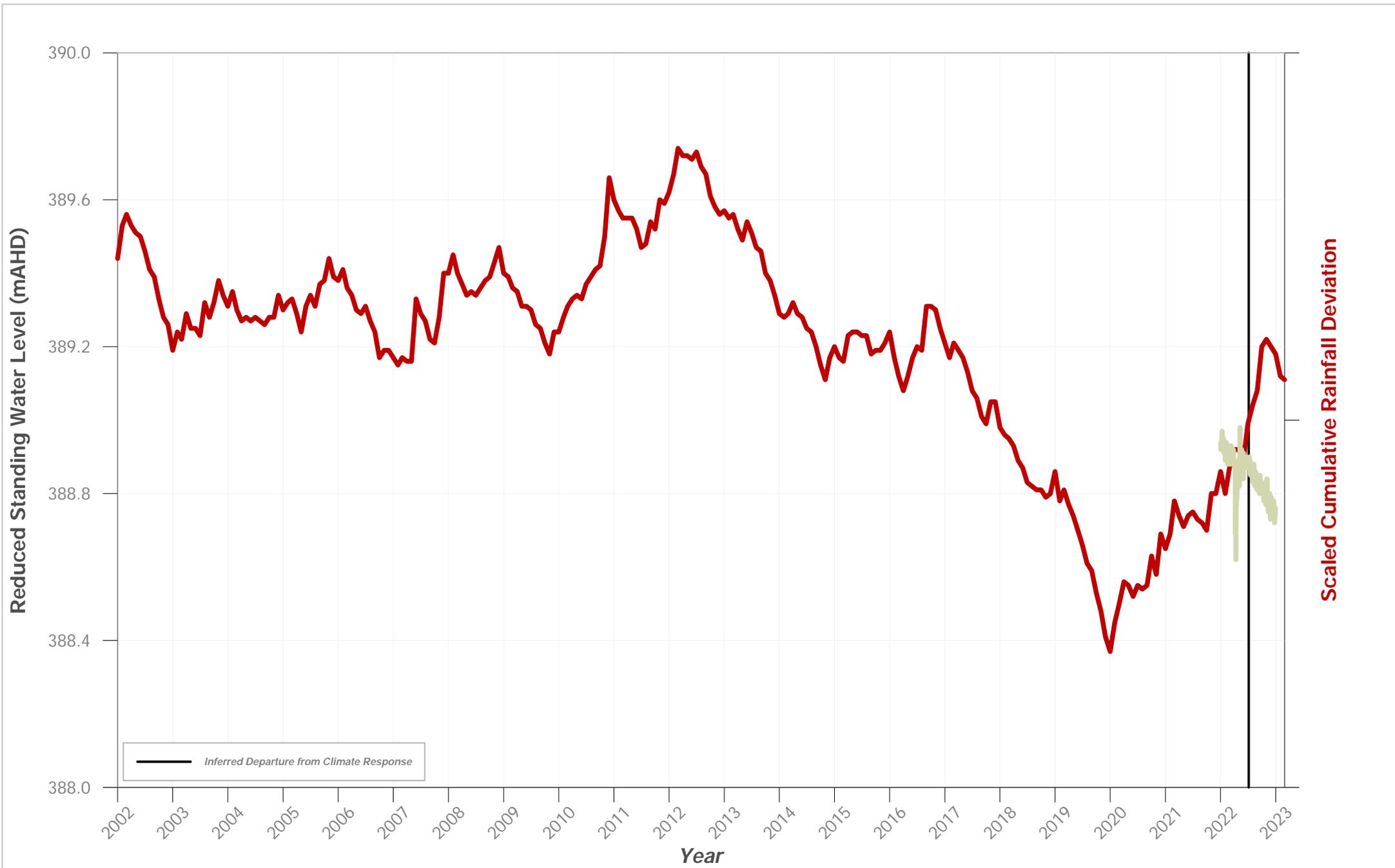
**Hydrograph of Groundwater Level Data for Bore ID: PZ 229 VWP 140m**
