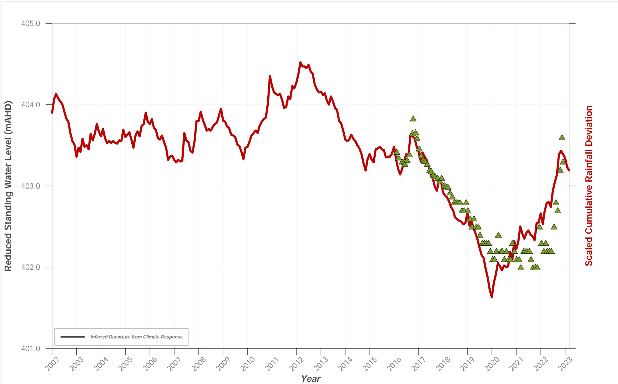
**Hydrograph of Groundwater Level Data for Bore ID: PZ 203**
