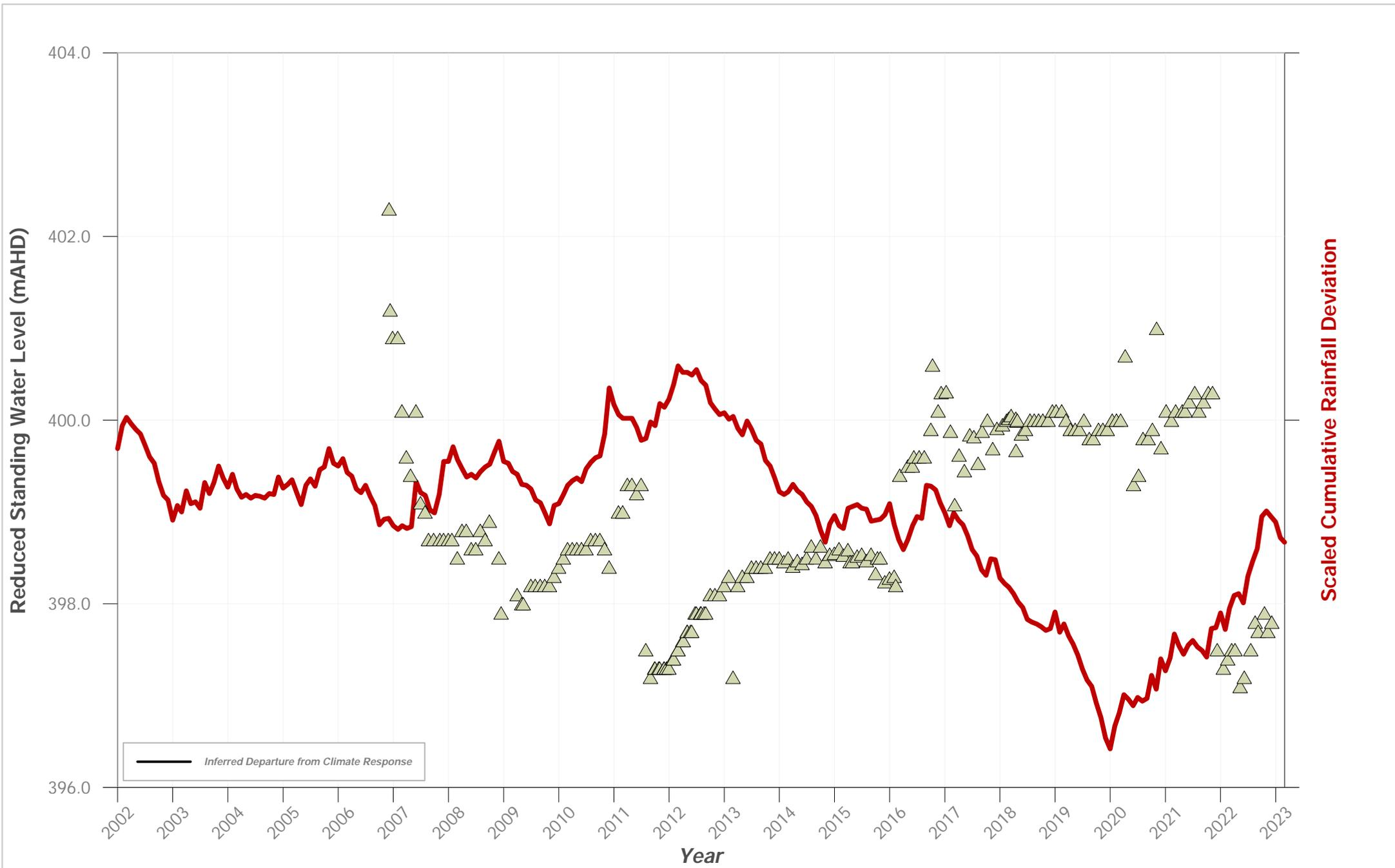
**Hydrograph of Groundwater Level Data for Bore ID: PZ 103C**
