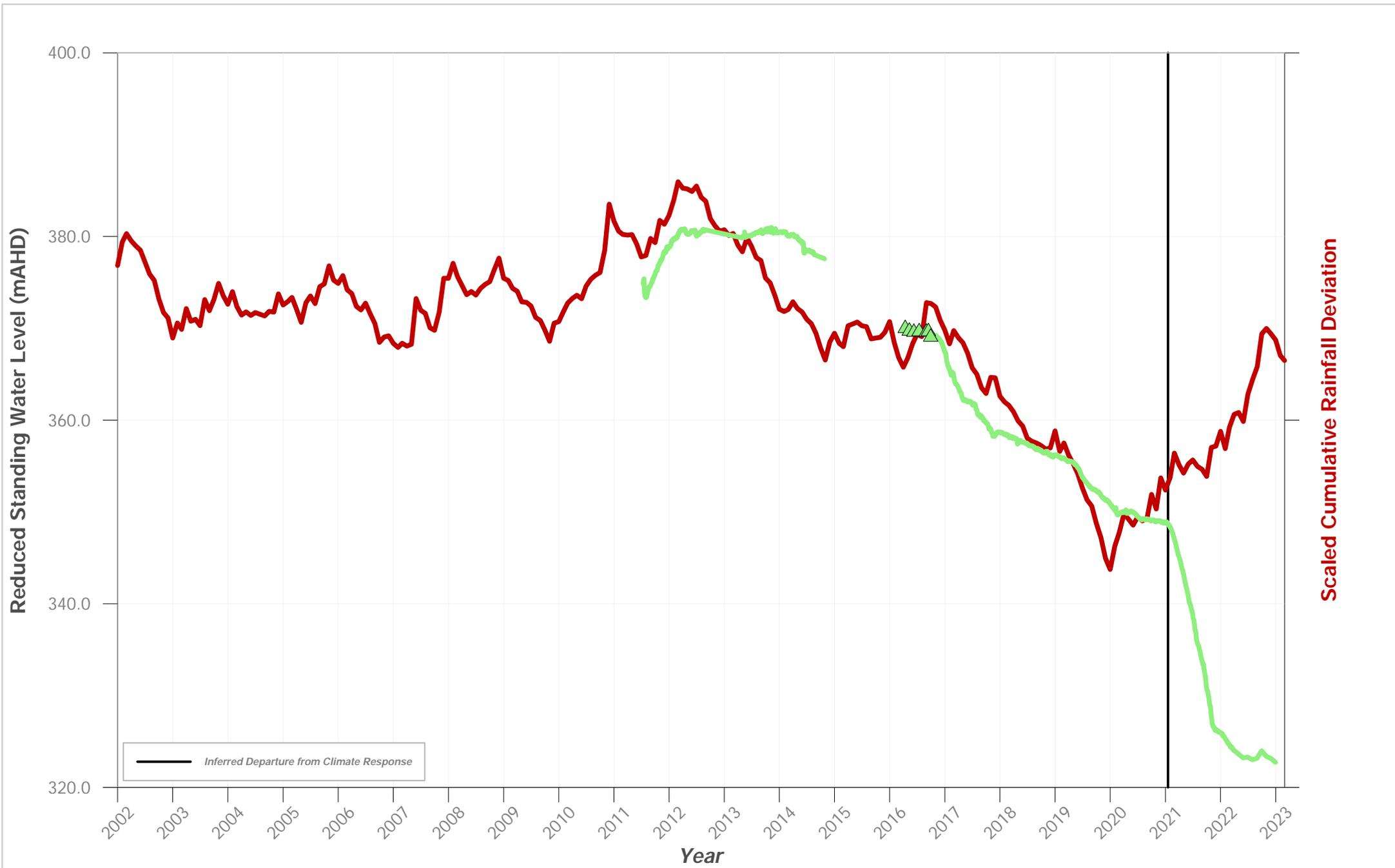
**Hydrograph of Groundwater Level Data for Bore ID: PZ 192 VWP 166m**
