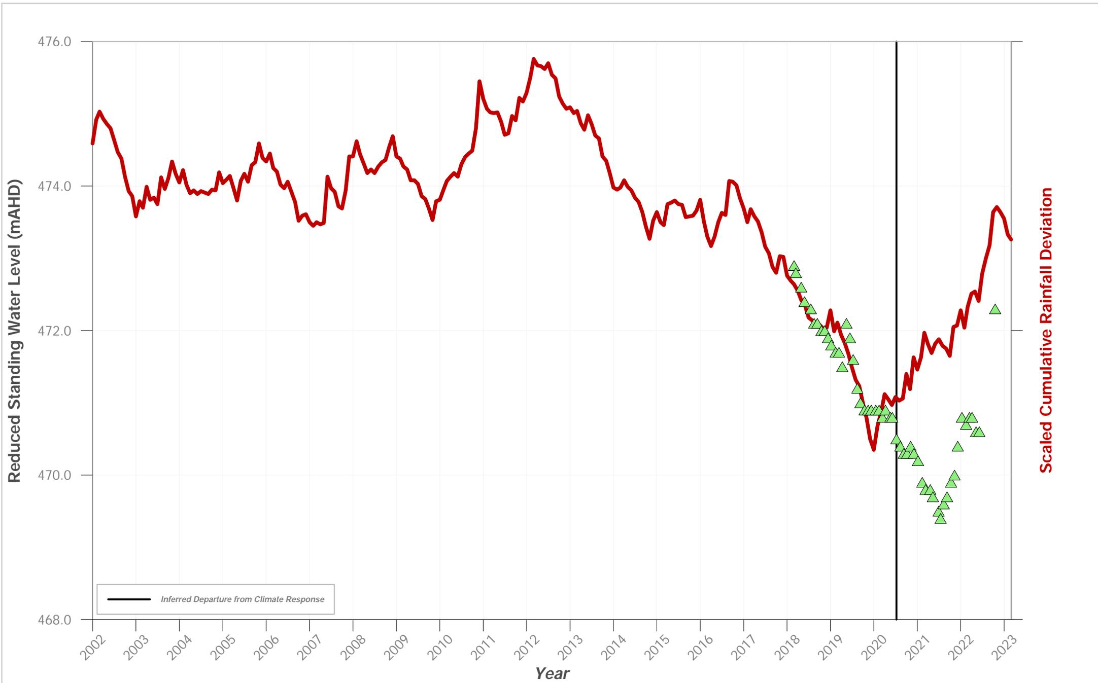
**Hydrograph of Groundwater Level Data for Bore ID: PZ 221**
