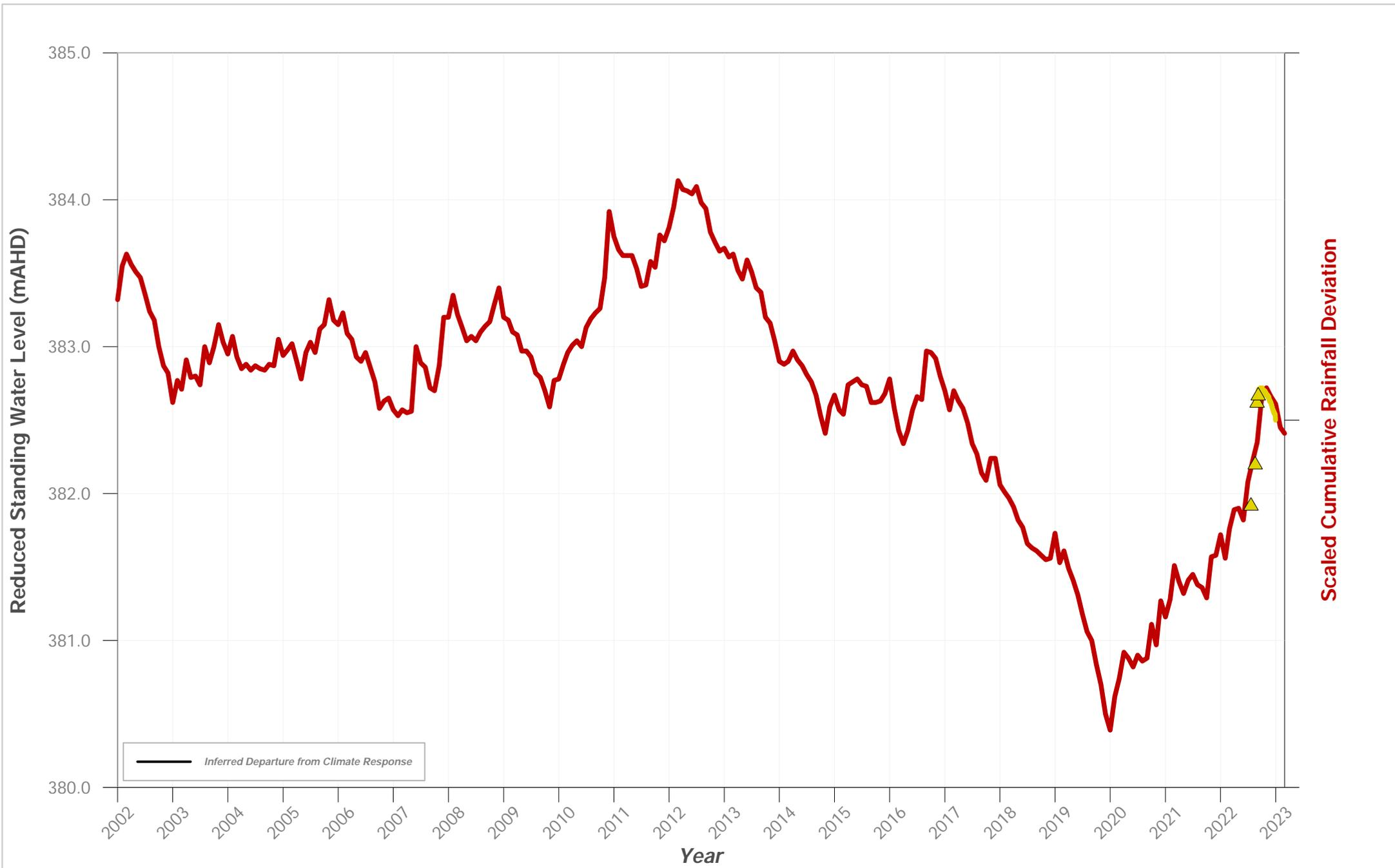
**Hydrograph of Groundwater Level Data for Bore ID: PZ 102C VWP 28m**
