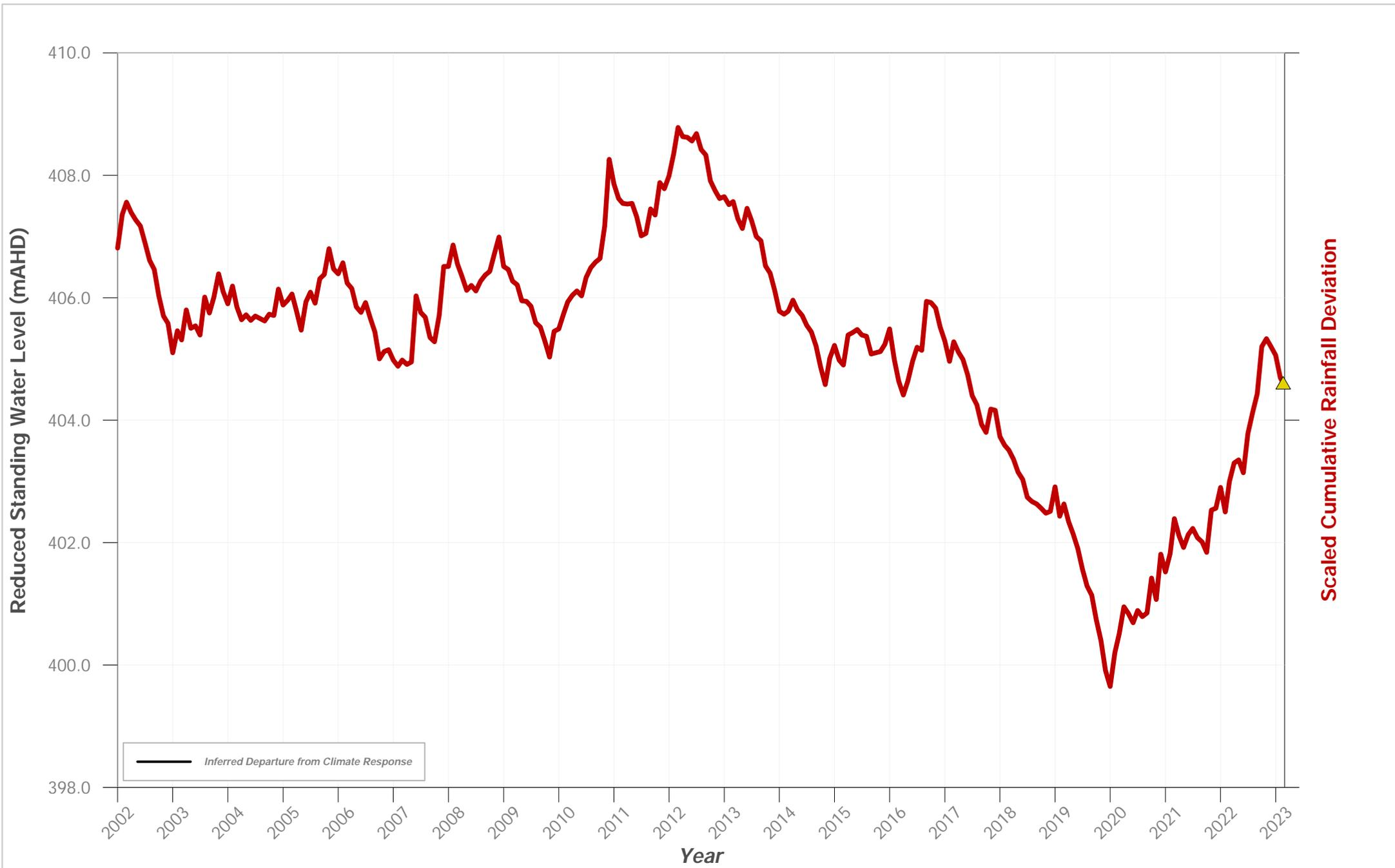
**Hydrograph of Groundwater Level Data for Bore ID: PZ 238 VWP 11m**
