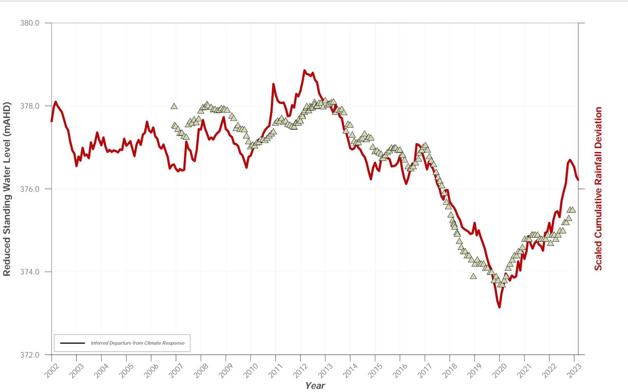
**Hydrograph of Groundwater Level Data for Bore ID: PZ 105C**
