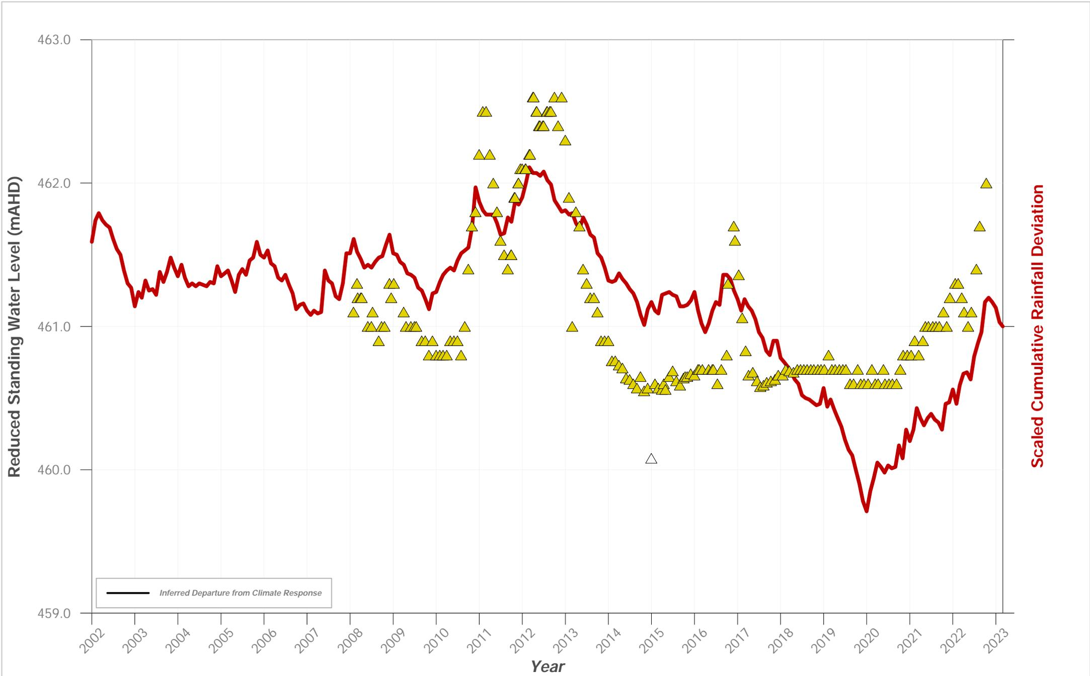
**Hydrograph of Groundwater Level Data for Bore ID: PZ 137**
