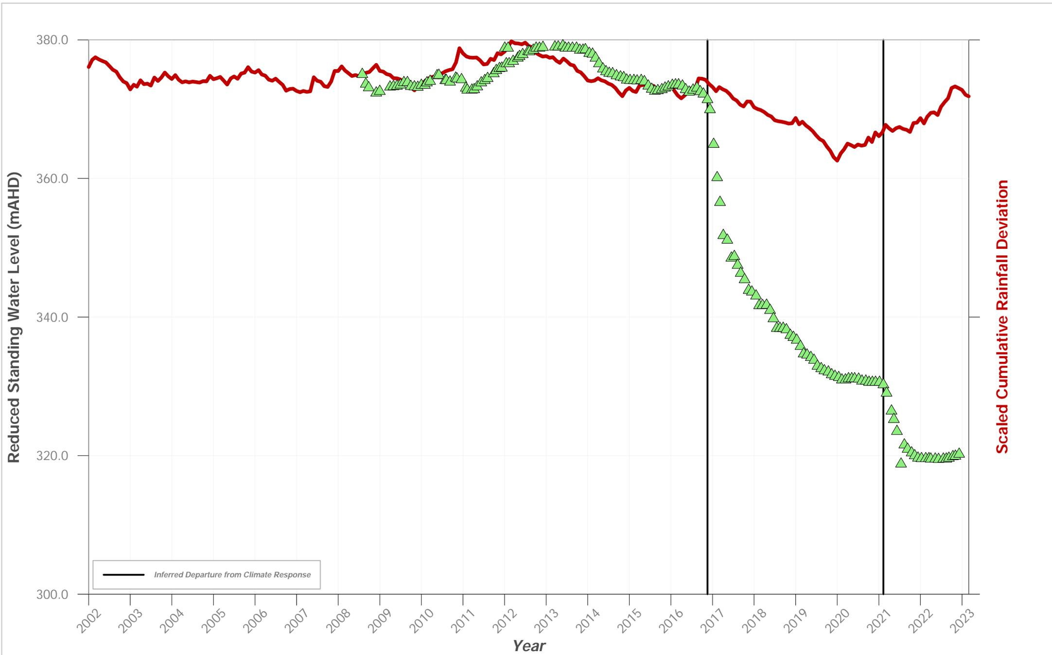
**Hydrograph of Groundwater Level Data for Bore ID: PZ 179 VWP 145m**
