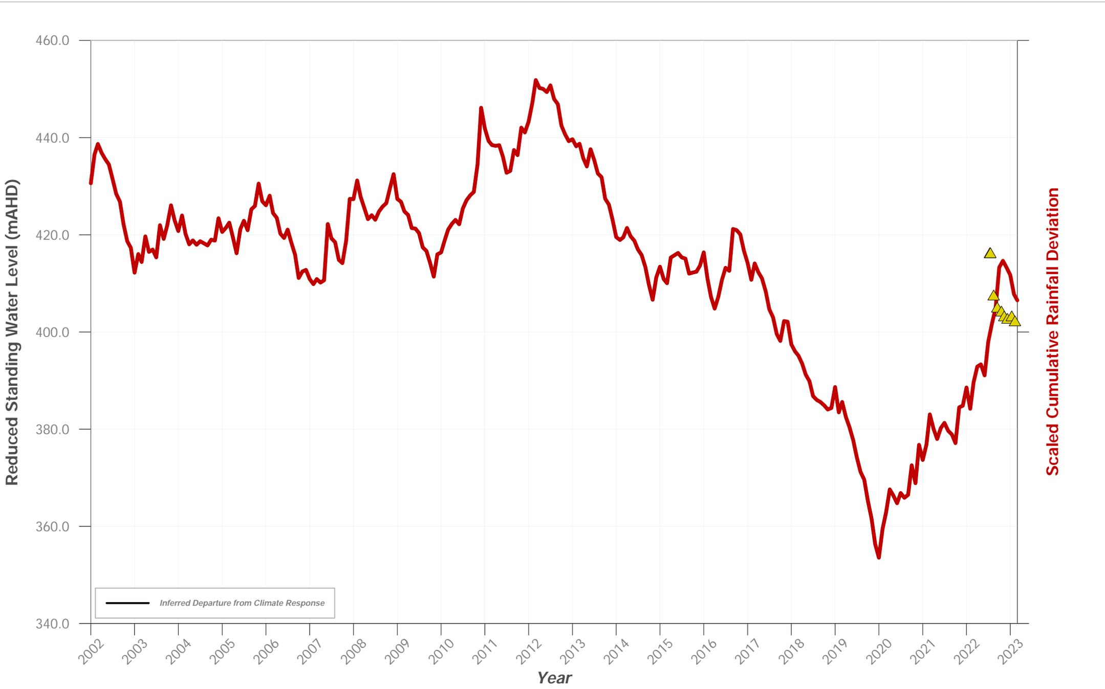
**Hydrograph of Groundwater Level Data for Bore ID: PZ 195C**
