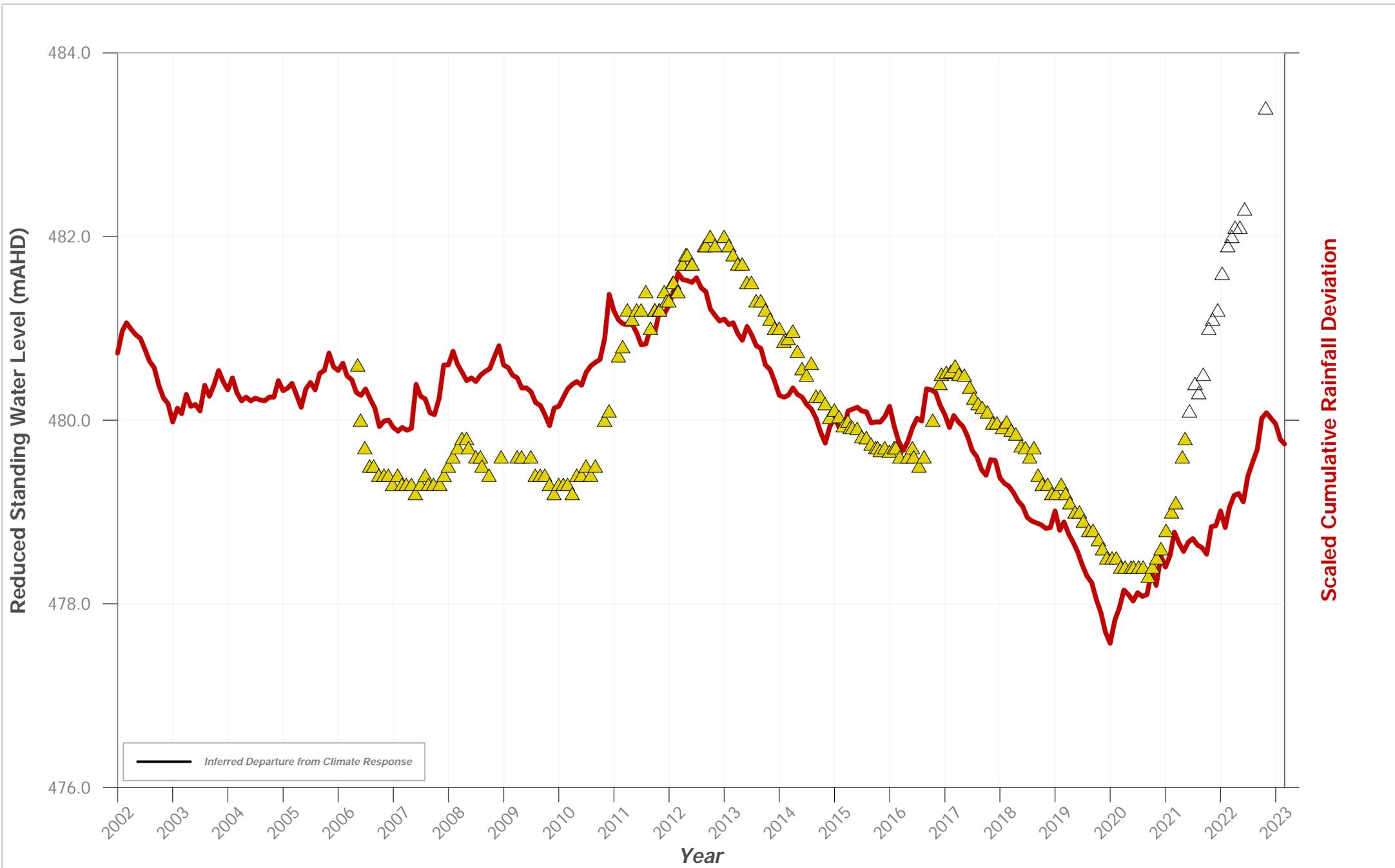
**Hydrograph of Groundwater Level Data for Bore ID: PZ 112B**
