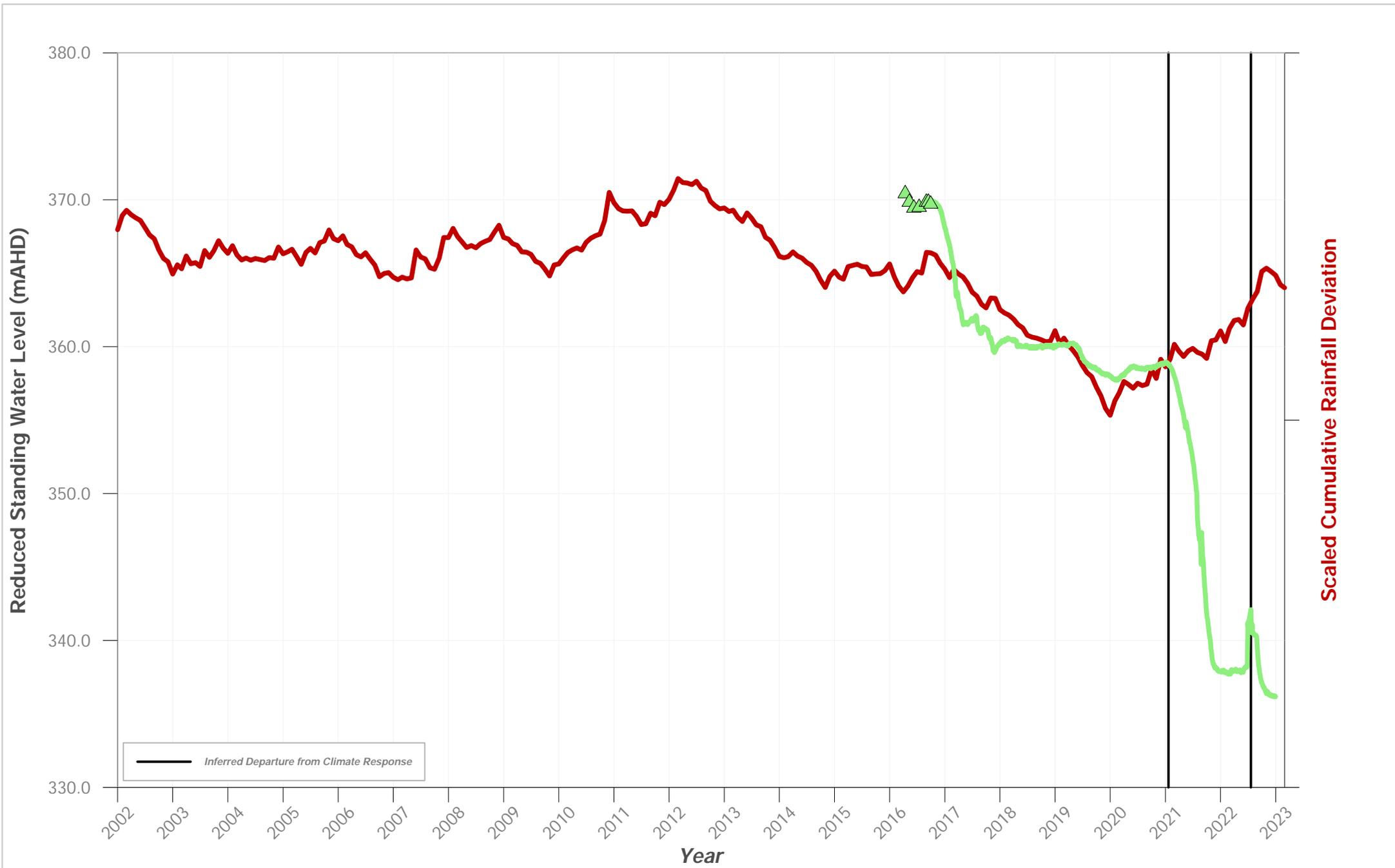
**Hydrograph of Groundwater Level Data for Bore ID: PZ 193 VWP 162m**
