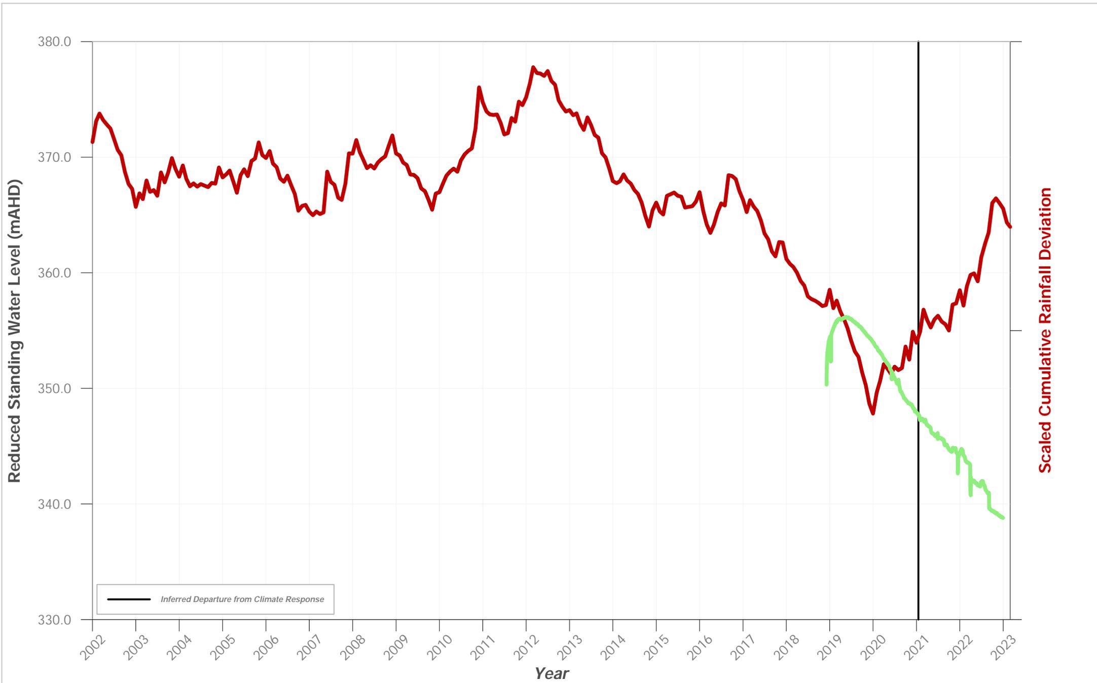
**Hydrograph of Groundwater Level Data for Bore ID: PZ 105A VWP 118m**
