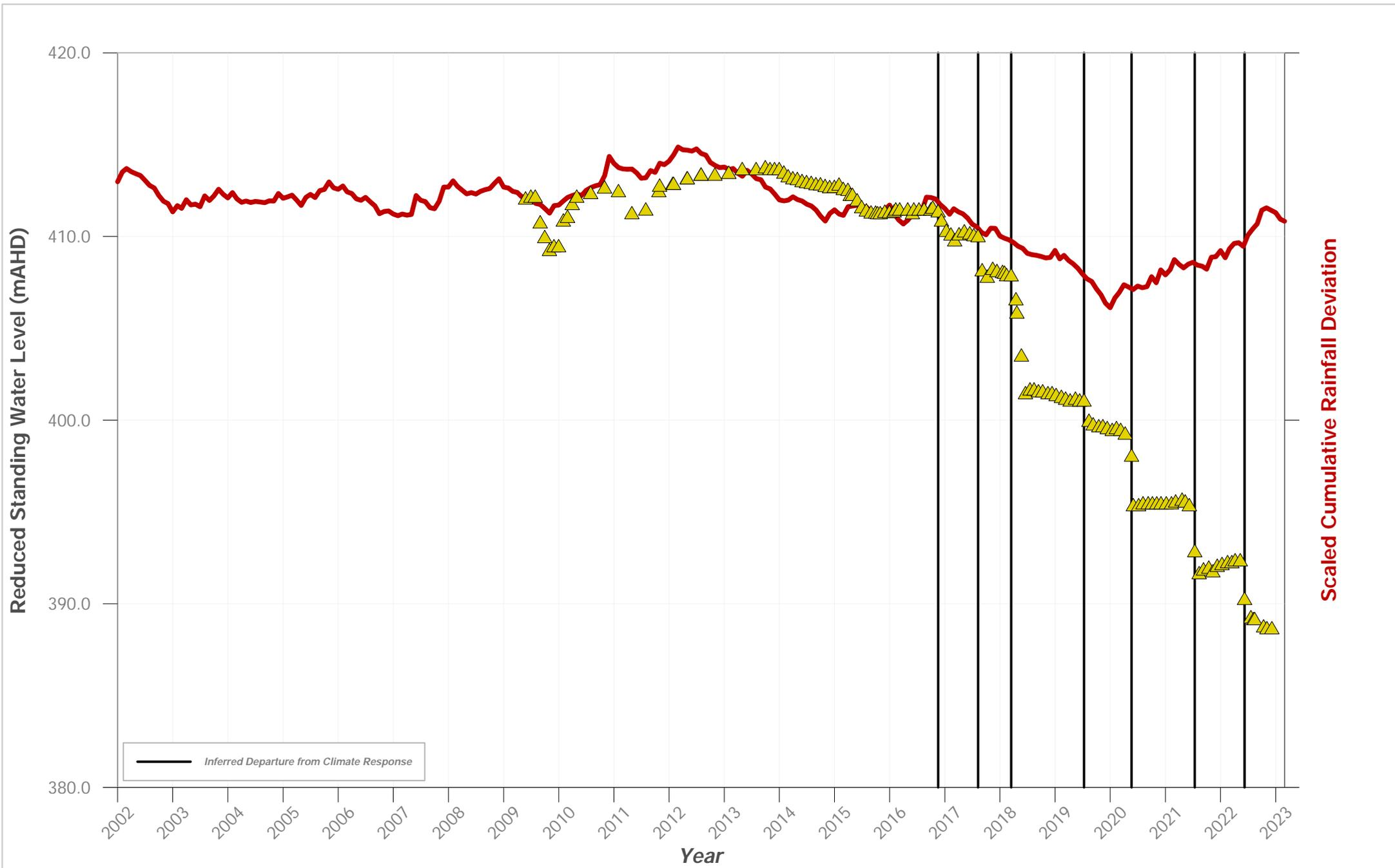
**Hydrograph of Groundwater Level Data for Bore ID: PZ 189**
