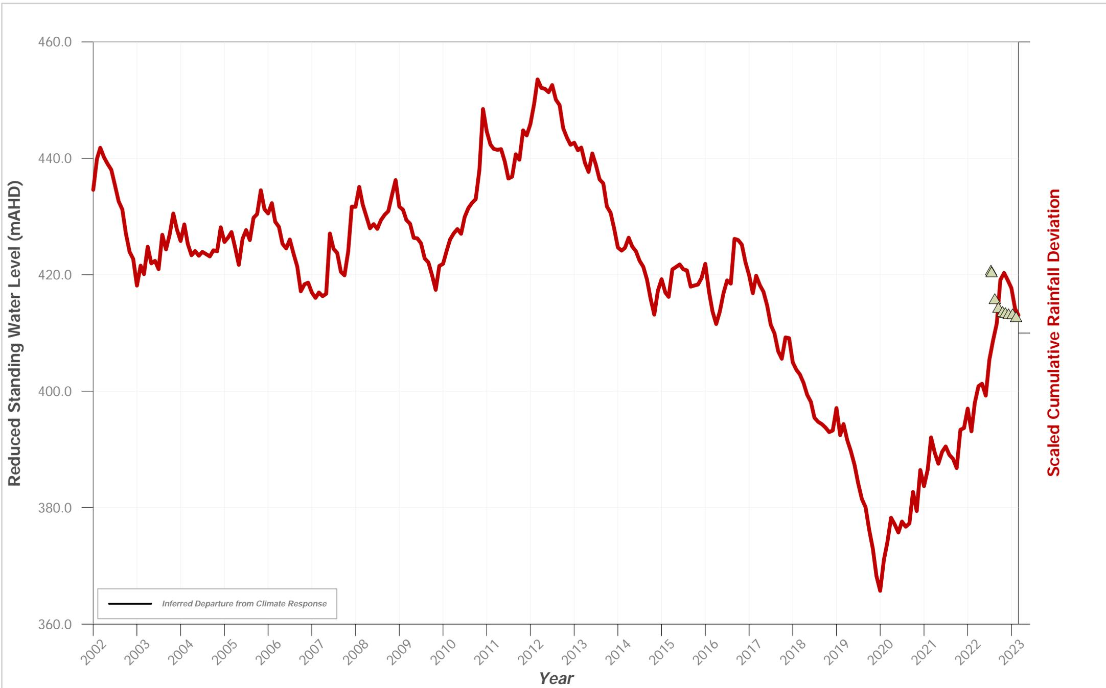
**Hydrograph of Groundwater Level Data for Bore ID: PZ 195B**
