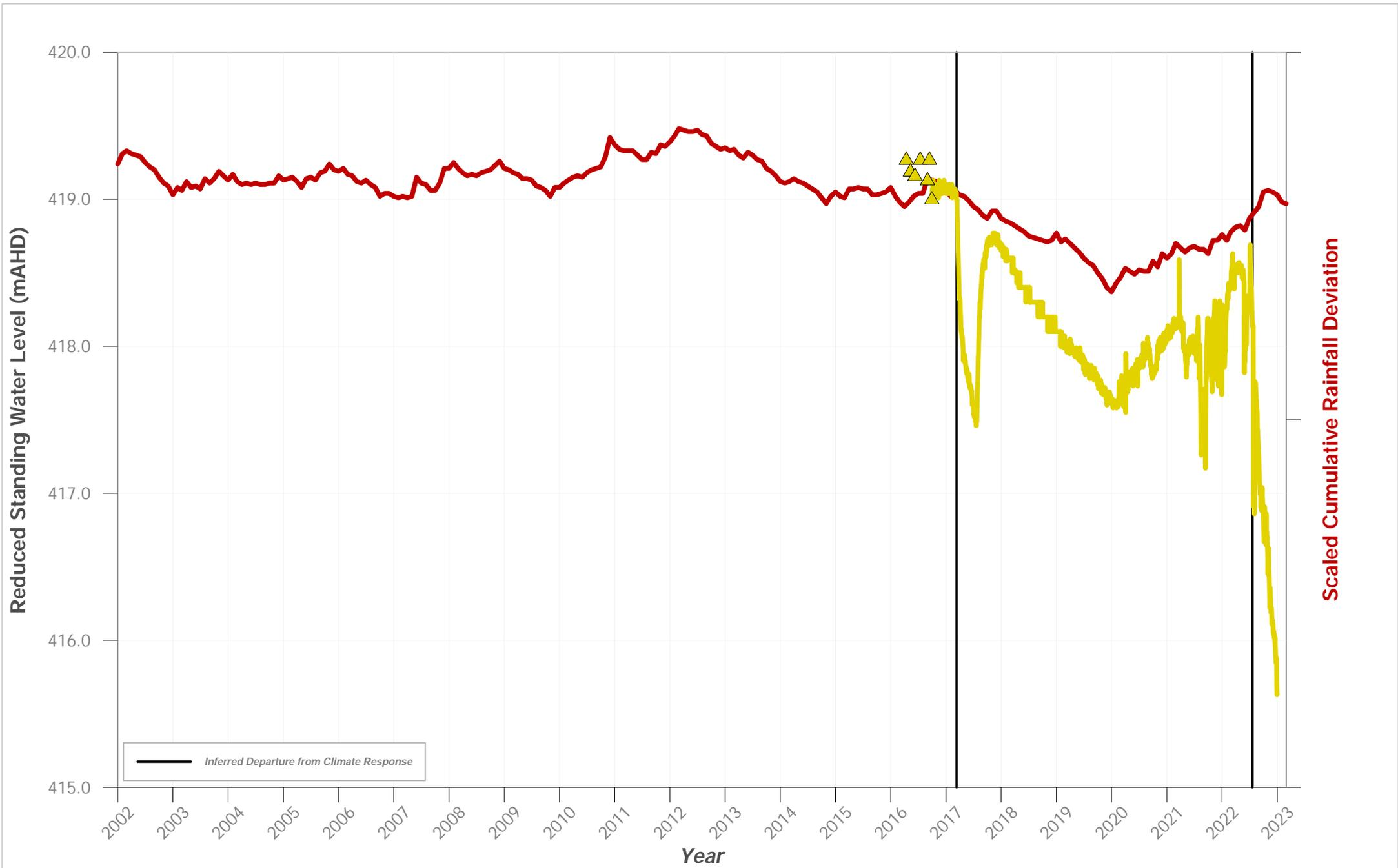
**Hydrograph of Groundwater Level Data for Bore ID: PZ 193 VWP 80m**
