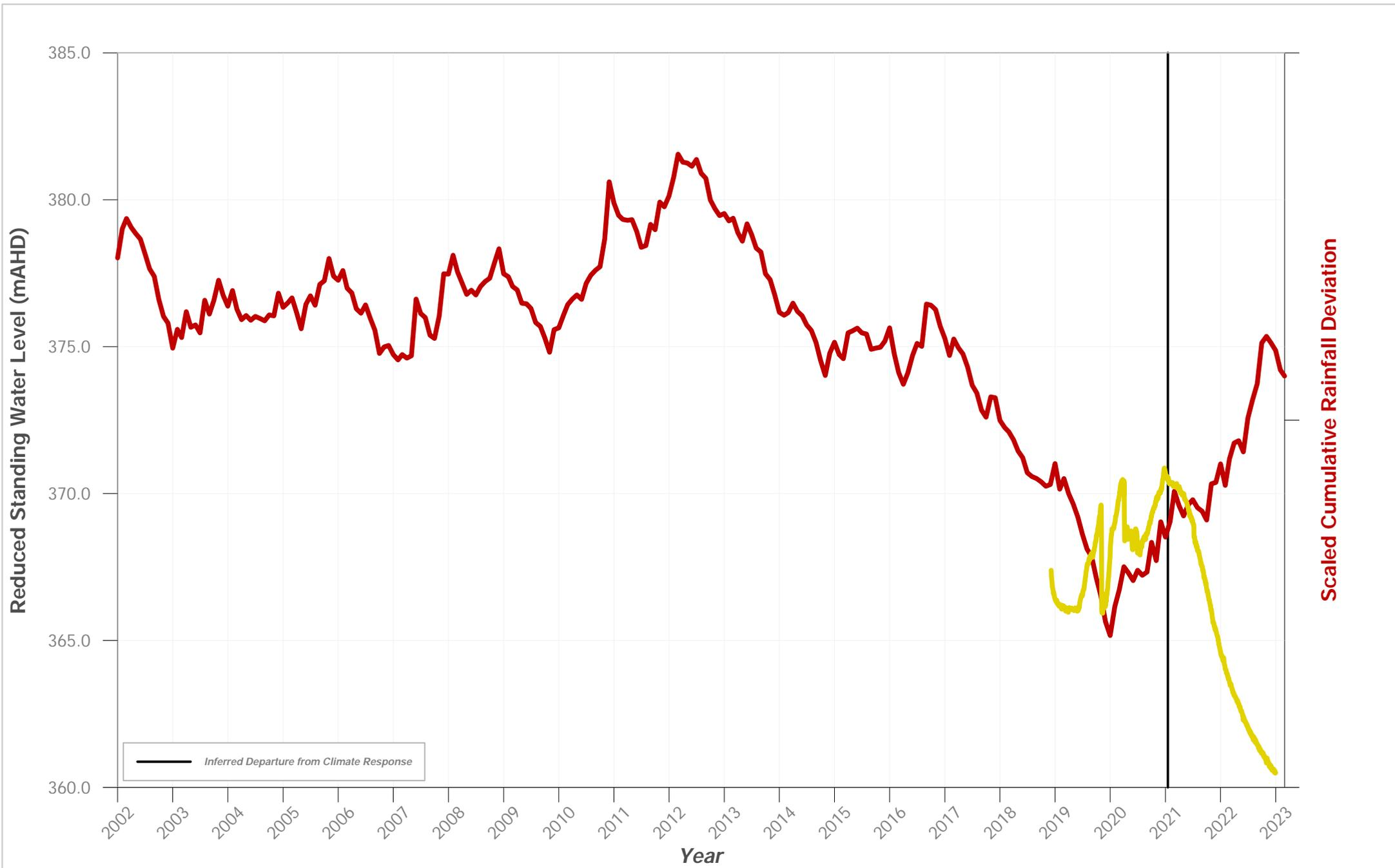
**Hydrograph of Groundwater Level Data for Bore ID: PZ 105A VWP 80m**
