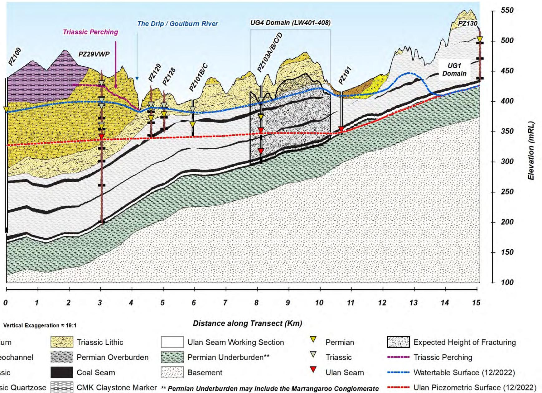
**Hydrogeological Conceptual Section B-B'** (refer to Figure 5.1 for Transect Location)
