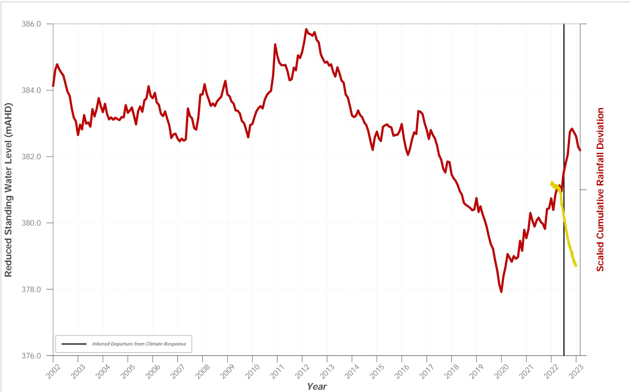
**Hydrograph of Groundwater Level Data for Bore ID: PZ 229 VWP 253m**
