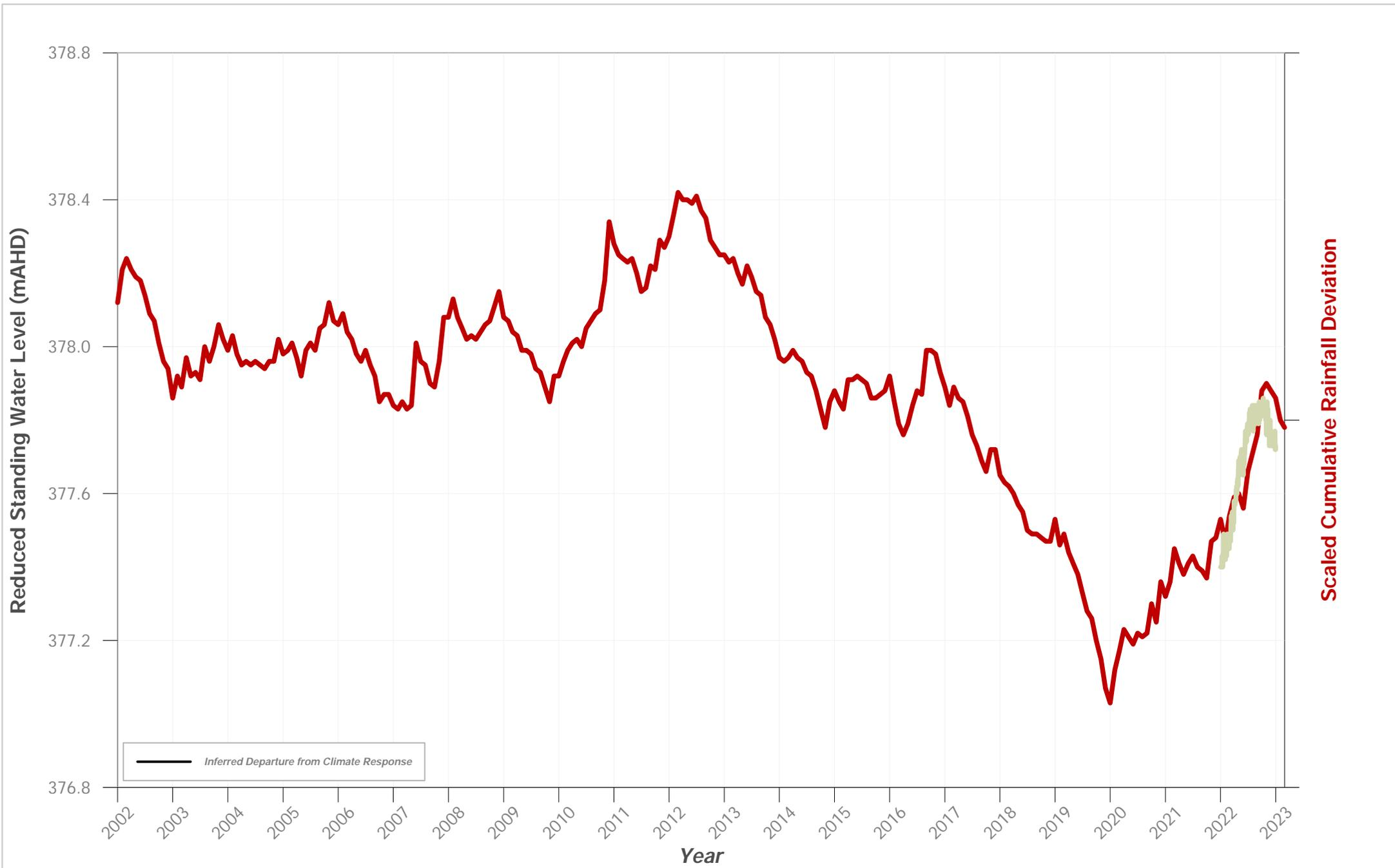
**Hydrograph of Groundwater Level Data for Bore ID: PZ 230 VWP 100m**
