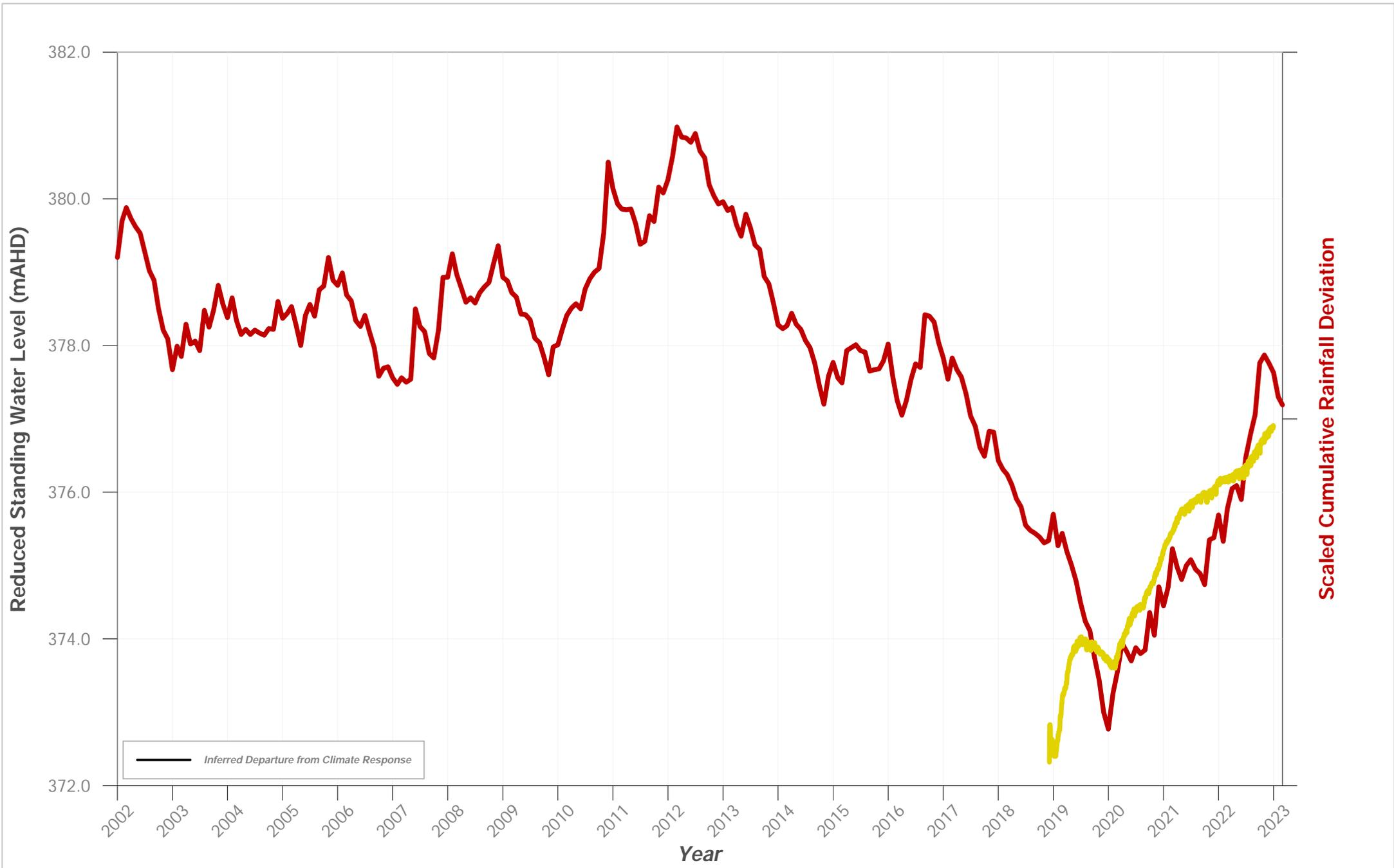
**Hydrograph of Groundwater Level Data for Bore ID: PZ 105A VWP 28m**
