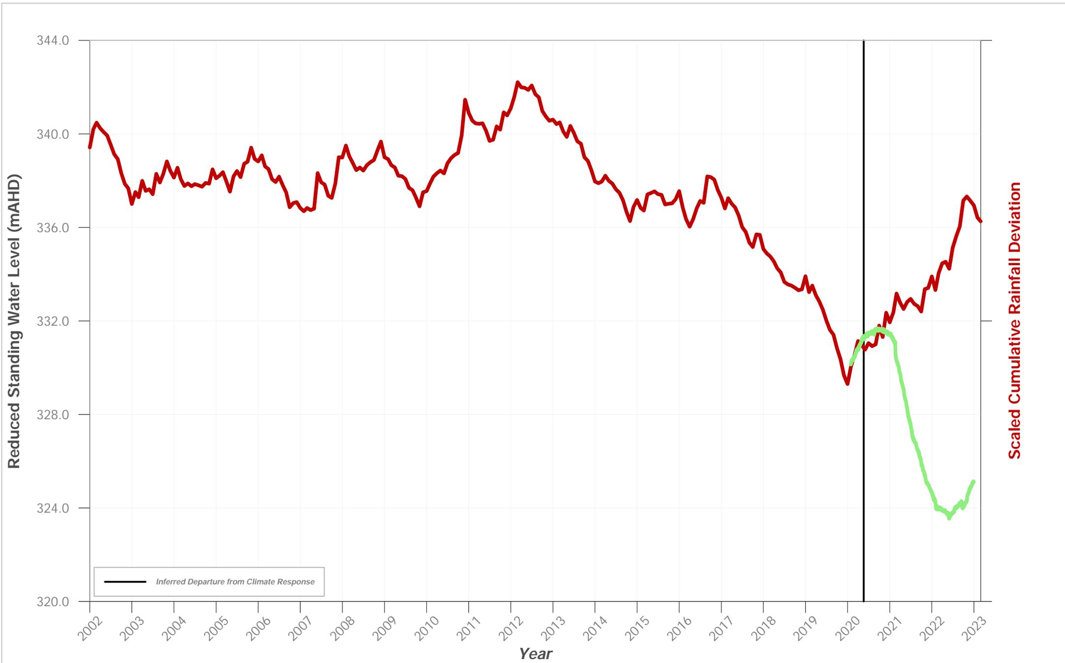
**Hydrograph of Groundwater Level Data for Bore ID: PZ 186 VWP 118m**
