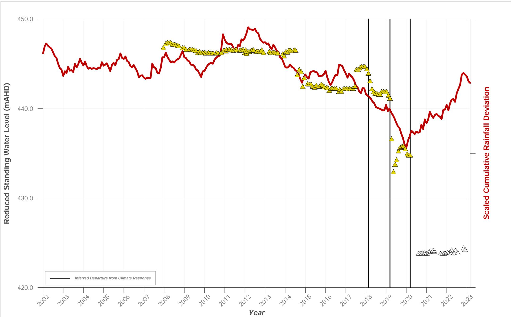
**Hydrograph of Groundwater Level Data for Bore ID: PZ 127 VWP 68m**
