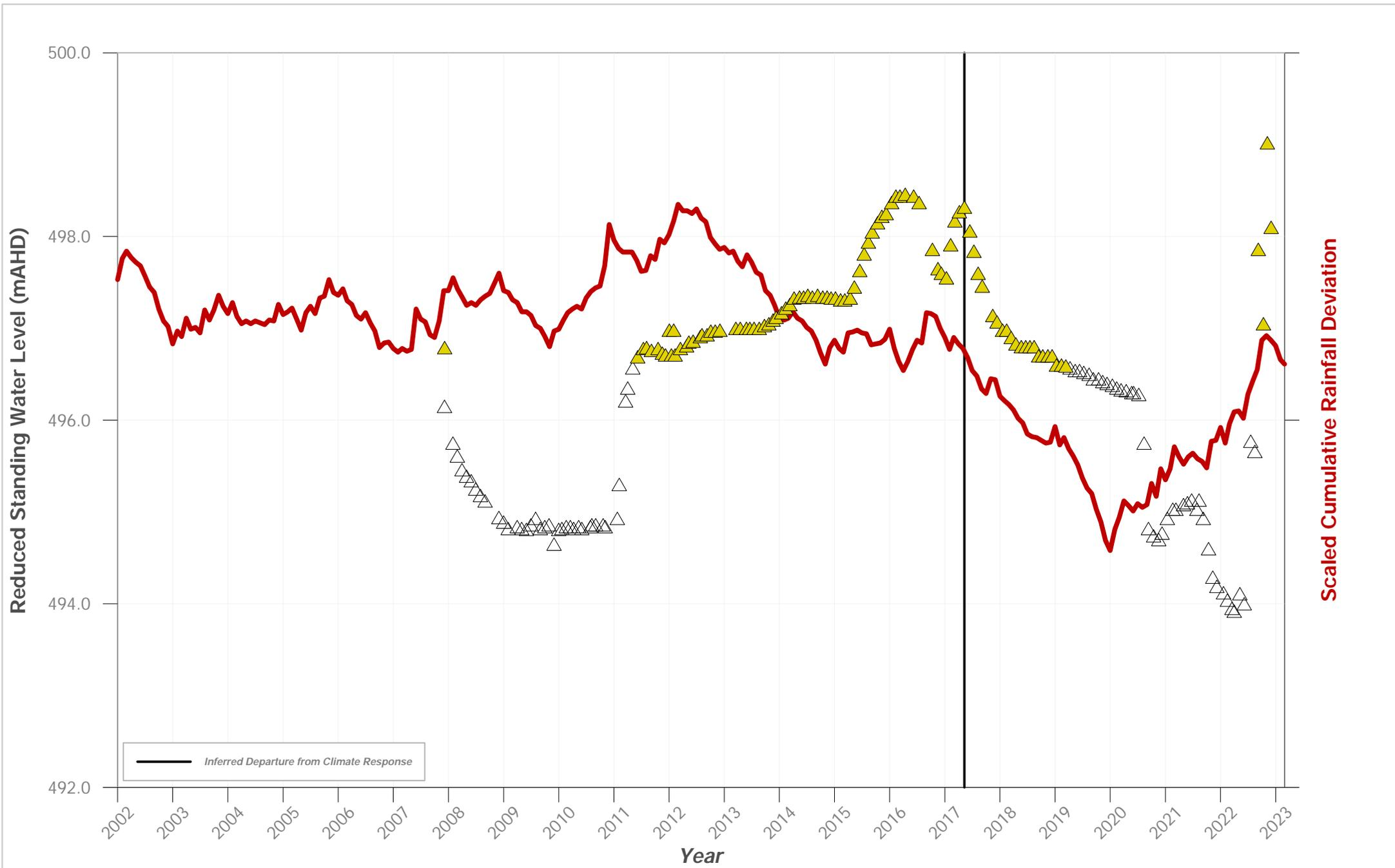
**Hydrograph of Groundwater Level Data for Bore ID: PZ 130 VWP 38.5m**
