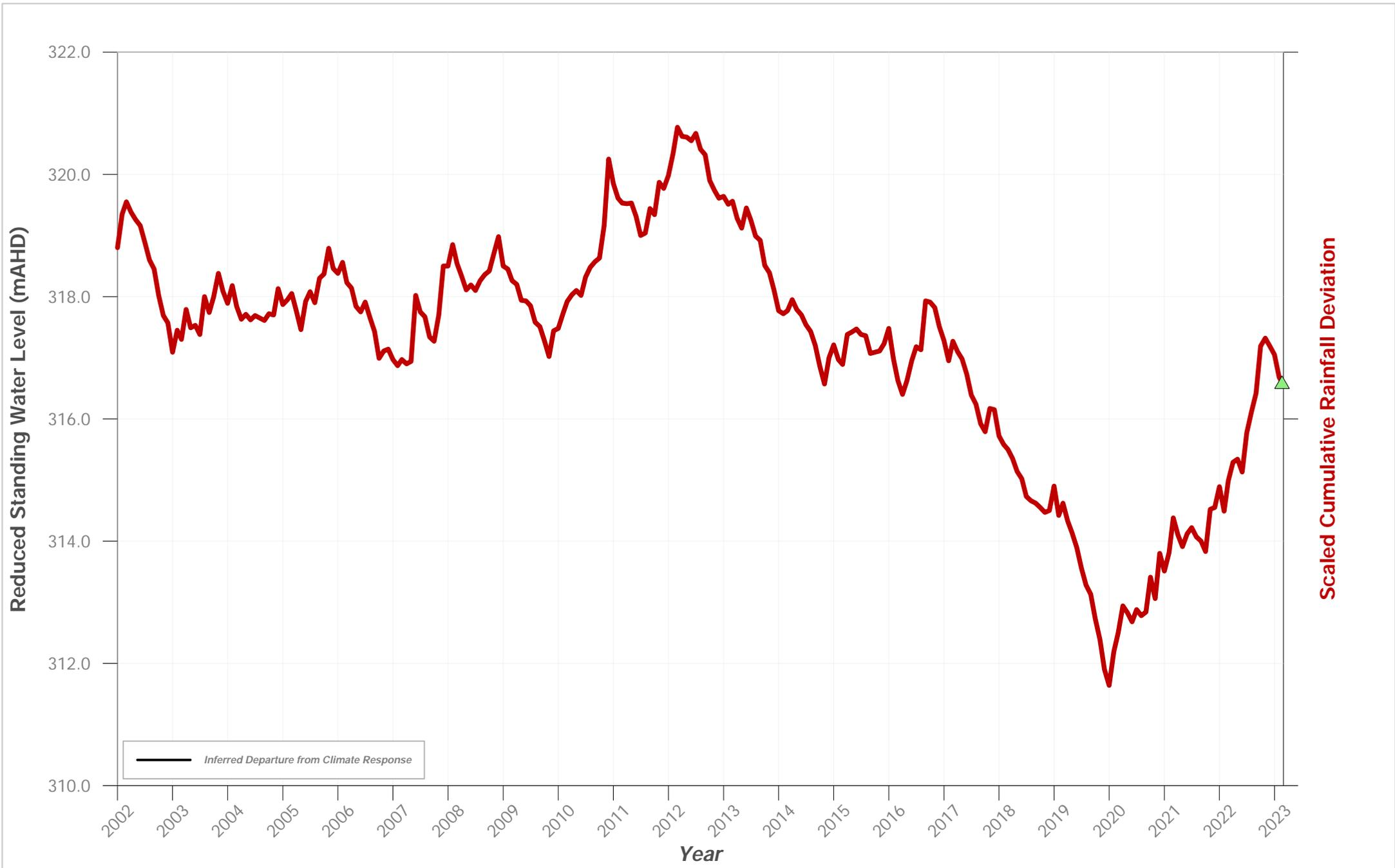
**Hydrograph of Groundwater Level Data for Bore ID: PZ 235B VWP 147m**
