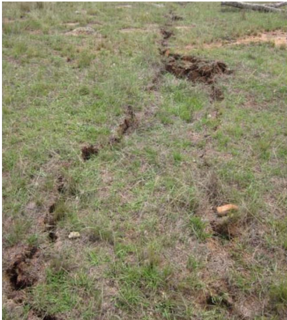
Fig. 4.10 Isolated Surface Cracking parallel to longwall tailgate above Longwall 26 at Ulan Coal Mine, 410m void width, 1.38m maximum observed subsidence, 240m cover (Ulan Longwall 26 End of Panel Subsidence Report)
