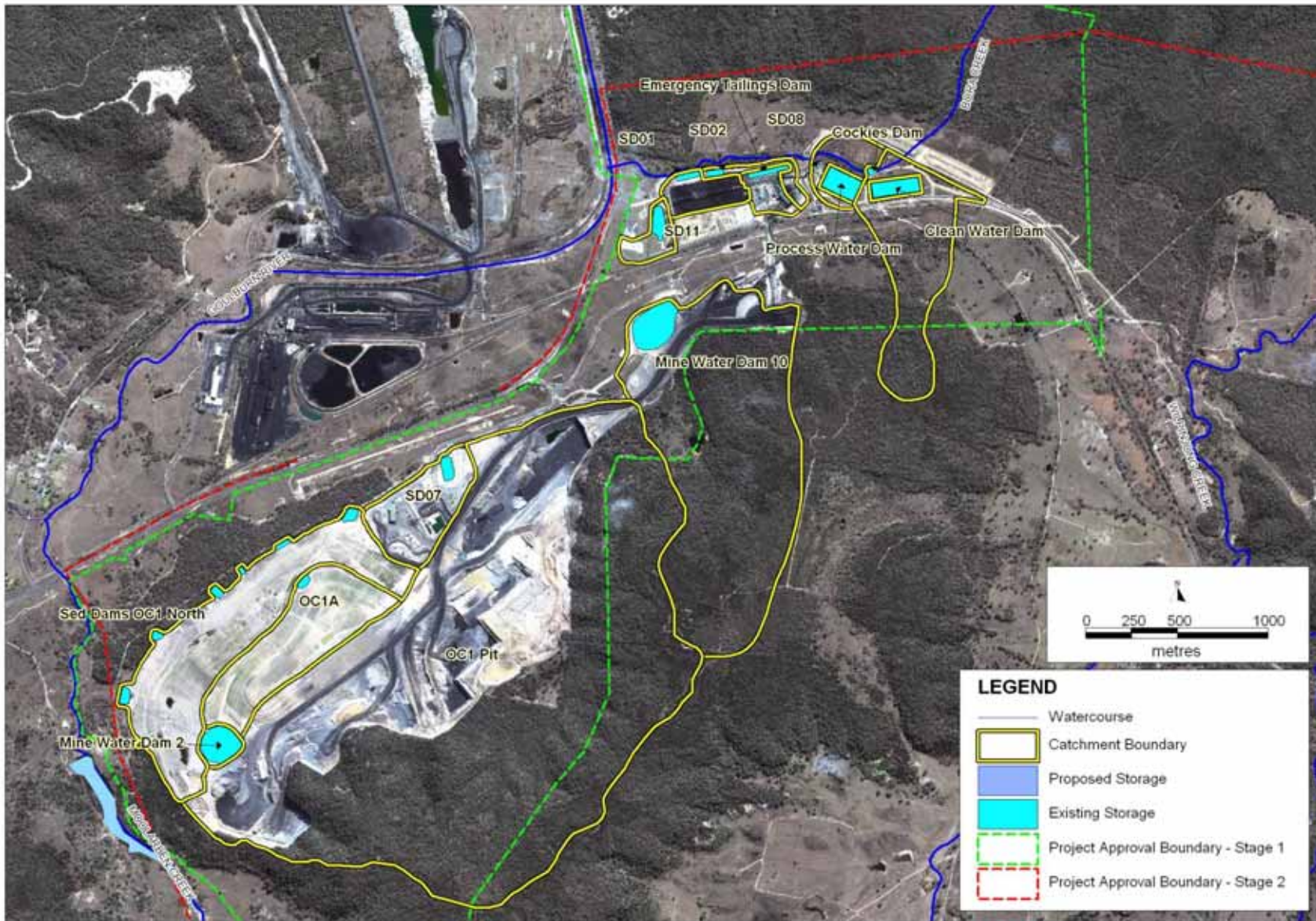
Figure 3.1 Location of Storages, Existing Water Management System
